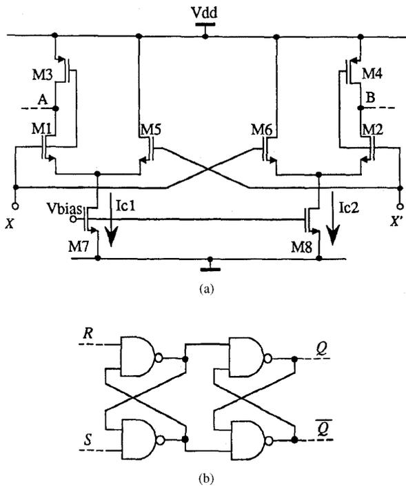
Fig. 2. Circuit implementation of (a) the ramp generator and (b) the feedback circuit.
