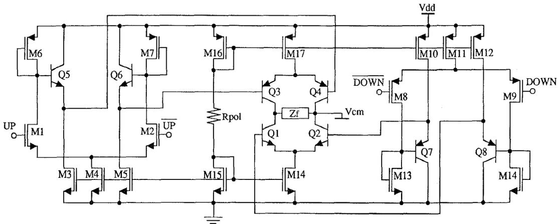
Fig. 5. Charge-pump circuit schematic.
