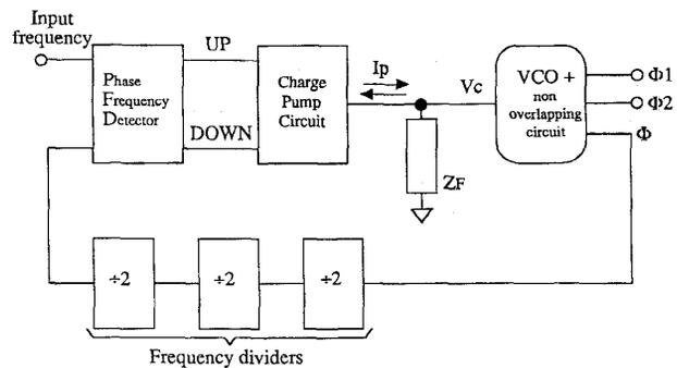
Fig. 4. Block schematic of the PLL.
