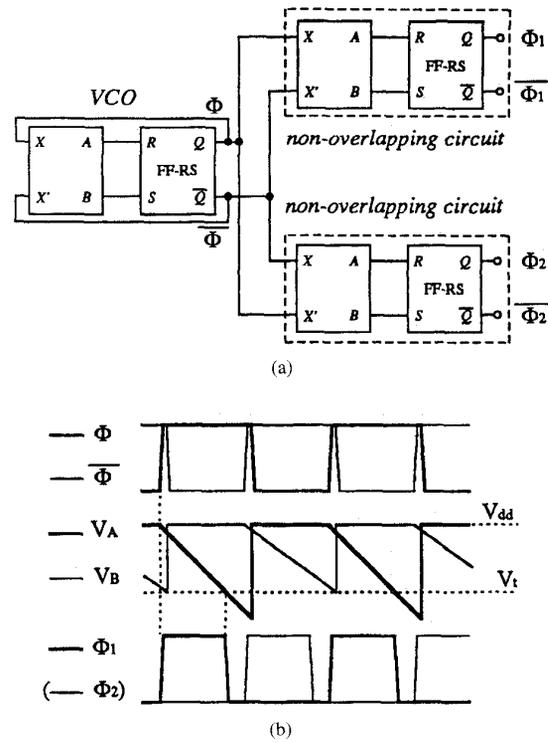
Fig. 3. (a) Overall block structure for the generation of the two nonoverlapping waveforms. (b) Corresponding voltage waveform  $V_A$  and  $\Phi_1$  ( $V_B$  and  $\Phi_2$  in thin lines).
