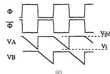
Fig. 1. (a) Ideal schematic of the ramp generation circuit. (b) Structure of the VCO. (c) Corresponding output waveforms.
