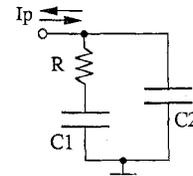
Fig. 6. Implementation of the loop impedance.
