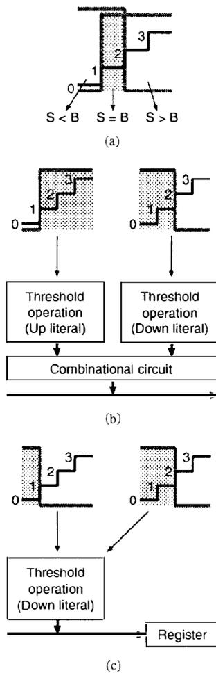
Fig. 2. Cell for four-valued one-digit comparison. (a) Principle of one-digit comparison. (b) Cell with two threshold elements. (c) Cell with one threshold element.
