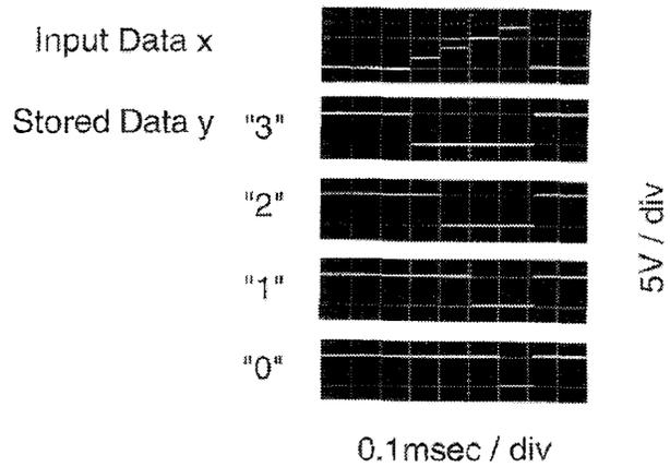
Fig. 7. Characteristics of an multiple-valued CAM cell.
