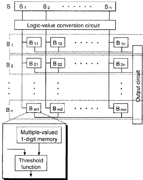
Fig. 1. Block diagram of a multiple-valued CAM.
