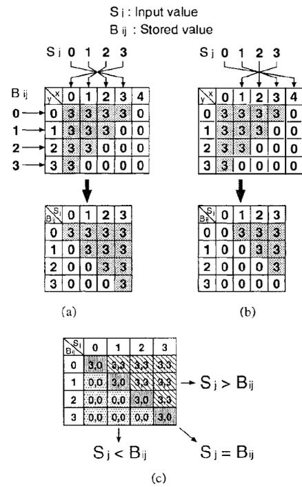
Fig. 3. Principle of four-valued one-digit comparison. (a) Step 1. (b) Step 2. (c) Comparison result.
