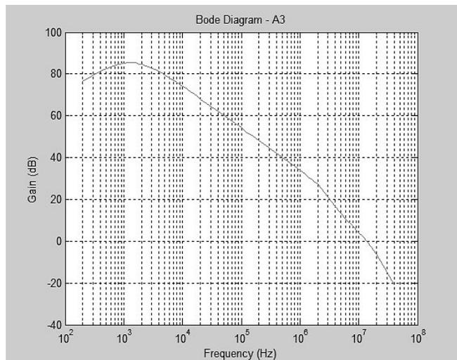
Figure 4 - Measured frequency response for the OTA Miller
