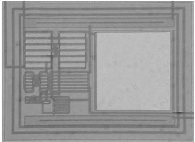
Figure 3 – Chip microphotography of the Miller OTA
