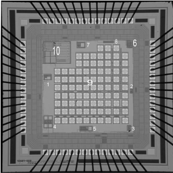
Figure 2 – AMS 0.35 $\mu\text{m}$  Test Chip microphotography
