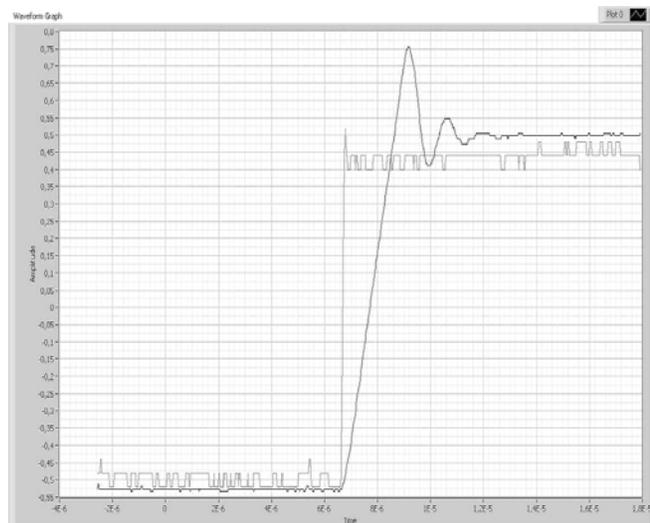
Figure 5 - Measured step response for the OTA Miller
