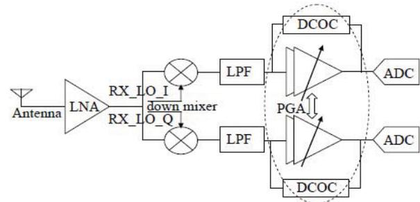
Fig. 1. Block diagram of the direct-conversion receiver
