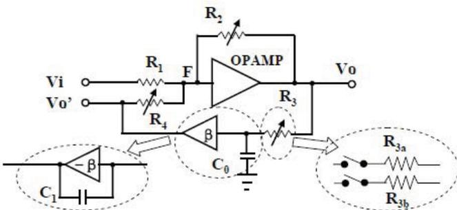
Fig. 7. Simplified architectures of stage1 and its DCOC loop
