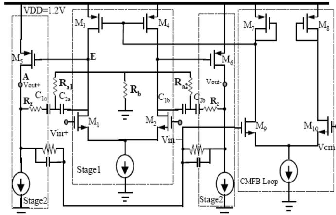
Fig. 4. Two-stage OPAMP with the proposed Miller Compensation.
