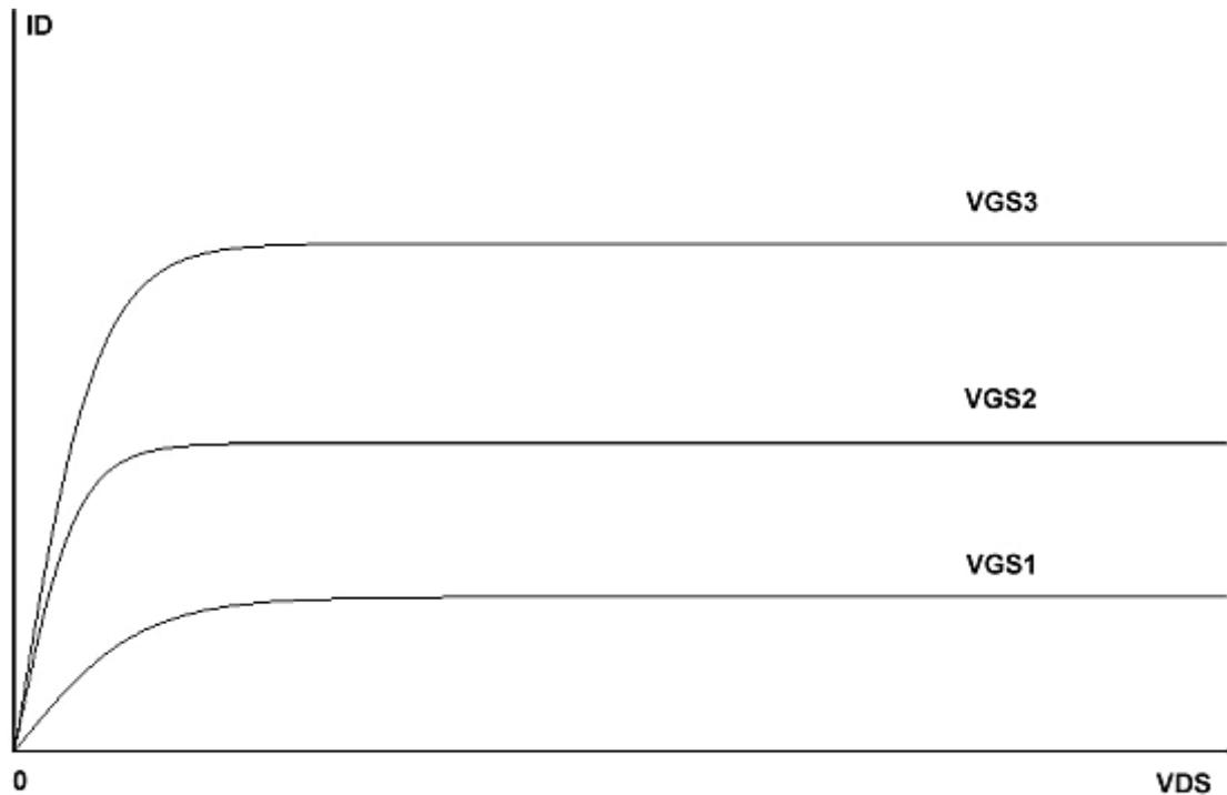
**Figure 1** A typical N-Channel FET I/V curve for different gate-to-source voltages, VGS1, VGS2, and VGS3.
