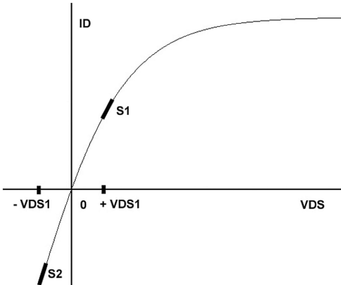
**Figure 2** FET's triode region extended to a negative VDS voltage, - VDS1, that still shows a resistance effect.
