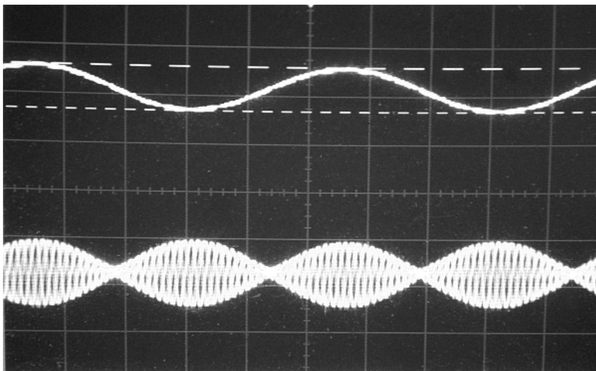
**Figure 22** Waveforms  $V_{mod}$  and  $V_{out}$  from Figure 21.
