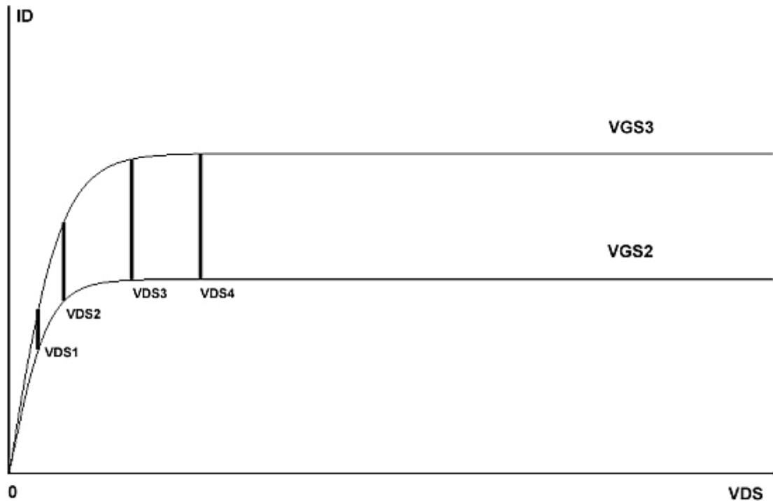
**Figure 24** The I V characteristics of an FET where a smaller VDS results in smaller change in drain current  $\Delta ID$  (as denoted by the thick vertical segments above VDS1 and VDS2 compared to vertical segments above VDS3 and VDS4) for the same change in gate to source voltage.
