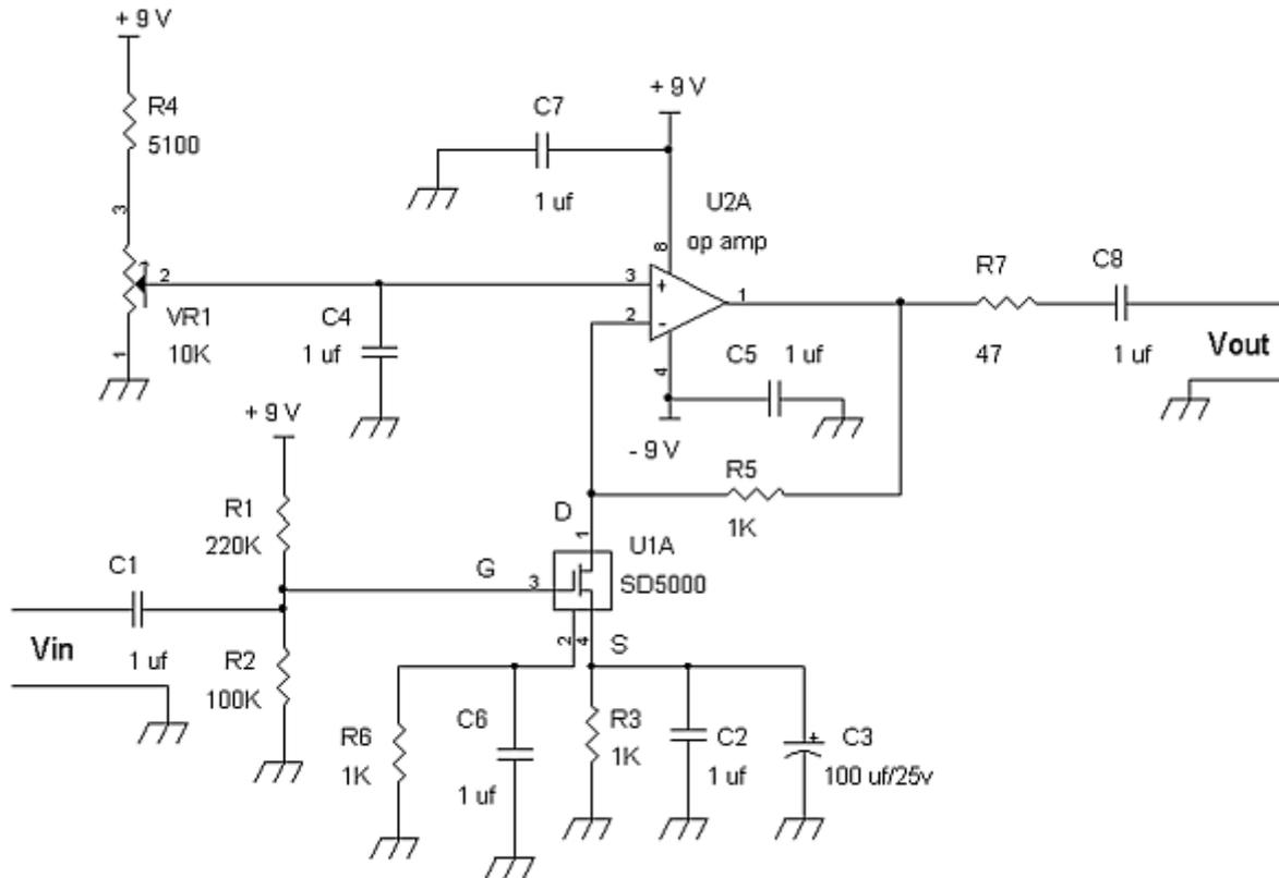
**Figure 25** A voltage controlled amplifier by varying the drain voltage of U1A.
