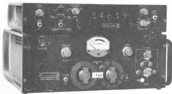
A 500-Mc Frequency Meter with High Sensitivity and Selectivity
