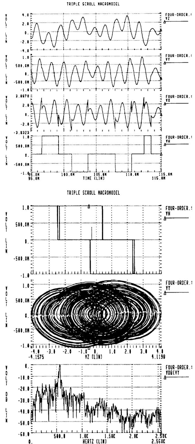
Fig. 5. Hspice simulation of 4-D chaotic oscillator.
