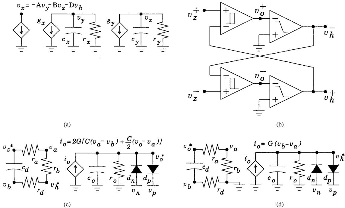
Fig. 2. Hspice models for 4-D chaotic oscillator. (a) Circuit model of quadrature-type oscillator. (b) Block diagram of differential hysteresis comparator. (c) Circuit model of hysteresis element. (d) Circuit model of comparator.
