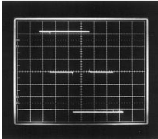
Fig. 12. Measured results from RC-opamp implementation:  $v_h(t)$  versus  $v_z(t)$ . The vertical axis is  $v_h(t)$  at 0.5 V/div and the horizontal axis is  $v_z(t)$  at 1 V/div.
