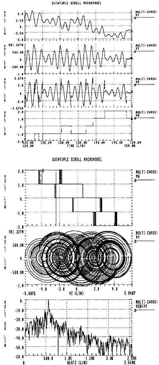
Fig. 7. Hspice simulation of 6-D chaotic oscillator.
