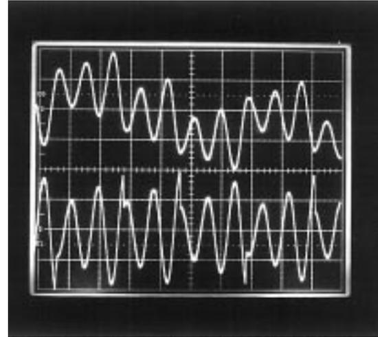
Fig. 10. Measured results from RC-opamp implementation: The top trace is  $v_z(t)$  at 2 V/div and the bottom trace is  $v_x(t)$  at 2 volts/div. Time scale is 2 ms/div.
