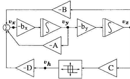
Fig. 1. Block diagram of 3-D tuned chaotic oscillator.
