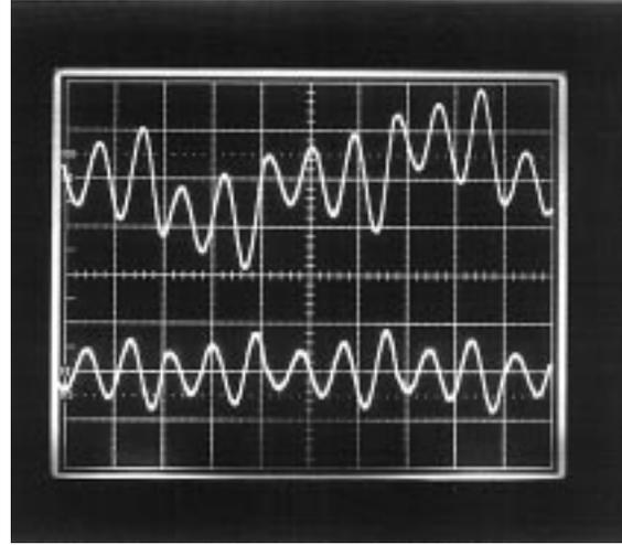
Fig. 9. Measured results from RC-opamp implementation: The top trace is  $v_z(t)$  at 2 volts/div and the bottom trace is  $v_y(t)$  at 1 V/div. Time scale is 2 ms/div.
