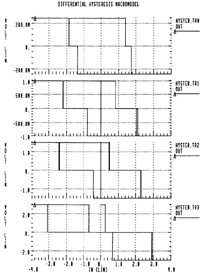
Fig. 3. Hspice simulations of macromodel of proposed hysteresis comparator for various output voltage limits. The horizontal axis is input voltage  $v_z(t)$  and the vertical axis is output voltage  $v_h(t)$ .
