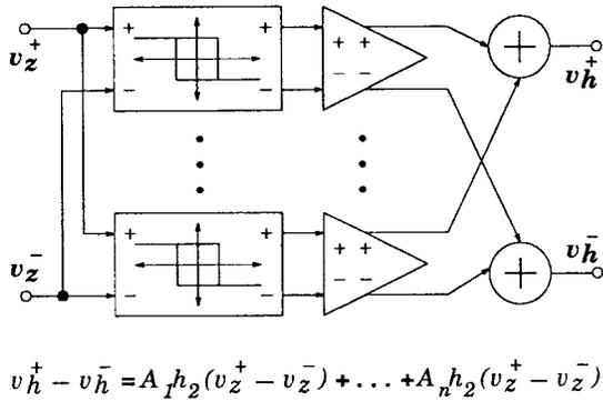
Fig. 6. Block diagram of design approach for higher order hysteresis.
