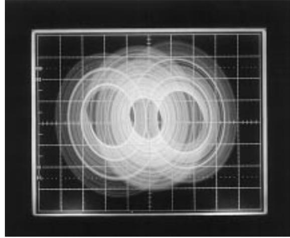
Fig. 13. Measured results from RC-opamp implementation:  $v_y(t)$  versus  $v_z(t)$ . The vertical axis is  $v_y(t)$  at 200 mV/div and the horizontal axis is  $v_z(t)$  at 1 V/div.
