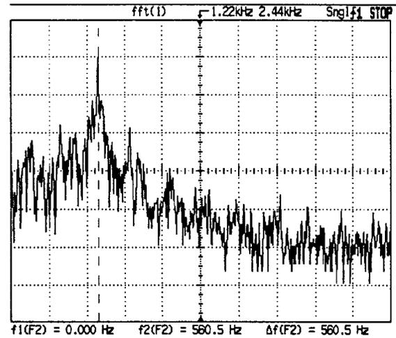
Fig. 14. Measured results from RC-opamp implementation: Frequency spectrum of  $v_y(t)$ .
