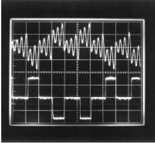
Fig. 11. Measured results from RC-opamp implementation: The top trace is  $v_z(t)$  at 2 V/div and the bottom trace is  $v_h(t)$  at 1 V/div. Time scale is 5 ms/div.
