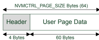
Figure 3-2. Internal Layout of an Emulated RWW EEPROM Page
