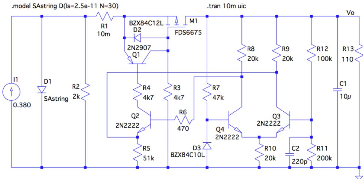
**Figure 1** Simple free-running photovoltaic voltage regulator (note: D2 & D3 are Zeners).
