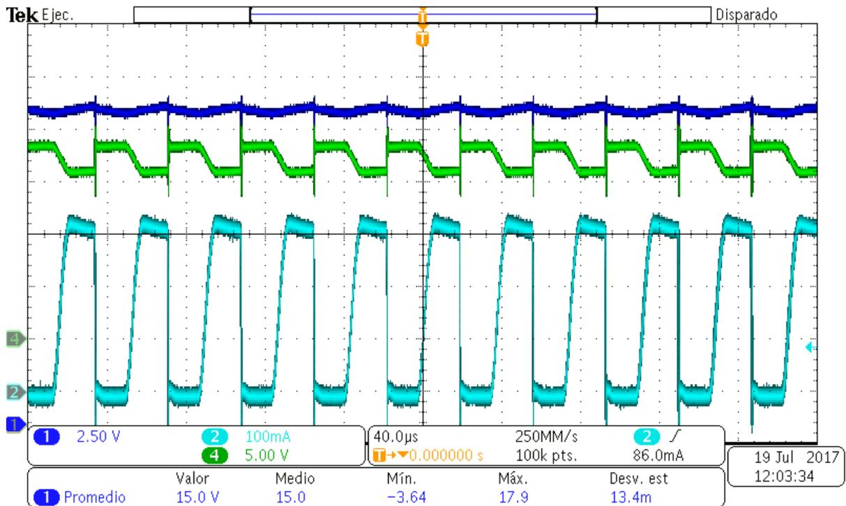
**Figure 2** Voltage regulator waveforms. Blue: output voltage; green: input voltage; cyan: M1 current.
