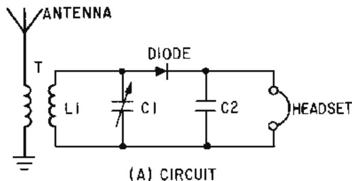
Figure 3-5A.—Series-diode detector and wave shapes. CIRCUIT.
