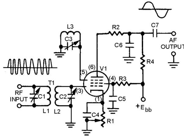
Figure 3-16.—Gated-beam detector.
