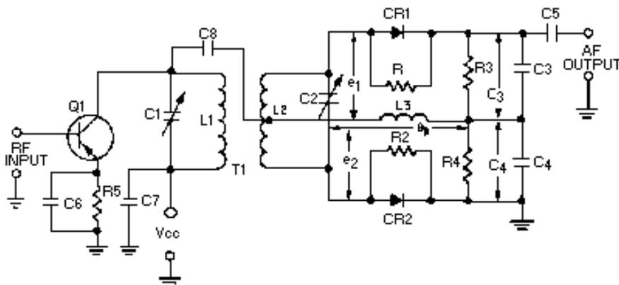
The **RATIO DETECTOR** uses a double-tuned transformer connected so that the instantaneous frequency variations of the fm input signal are converted into instantaneous amplitude variations.
