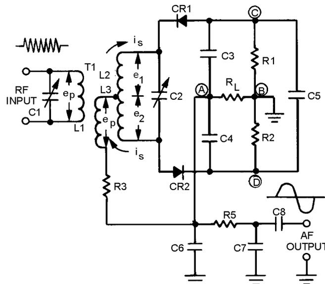
Figure 3-12.—Ratio detector.
