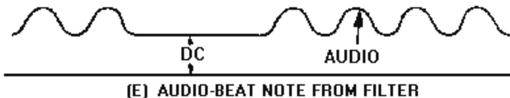
Figure 3-3E.—Heterodyne detection. AUDIO-BEAT NOTE FROM FILTER.
