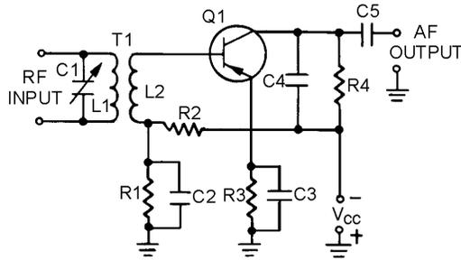
The **COMMON-BASE DETECTOR** is an amplifying detector that is used in portable receivers.
