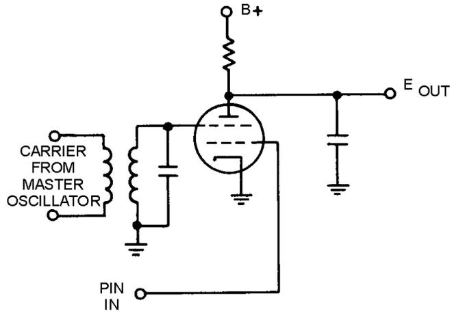
Figure 3-19.—Phase detector.
