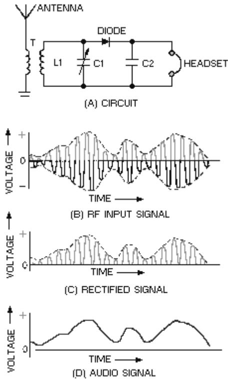
**SHUNT- (CURRENT-) DIODE DETECTOR** is characterized by a rectifier diode in parallel with the input and load impedance.
