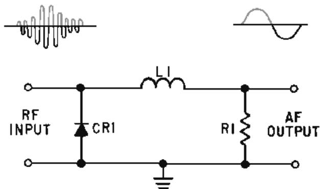
Figure 3-6.—Shunt-diode detector.
