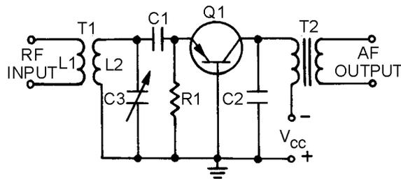
The **SLOPE DETECTOR** is the simplest form of frequency detector. It is essentially a tank circuit tuned slightly away from the desired fm carrier.
