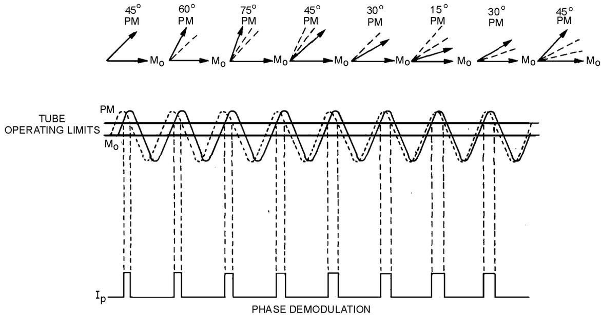
Figure 3-20.—Phase-detector waveforms.
