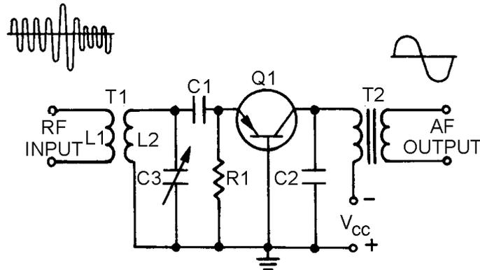
Figure 3-8.—Common-base detector.
