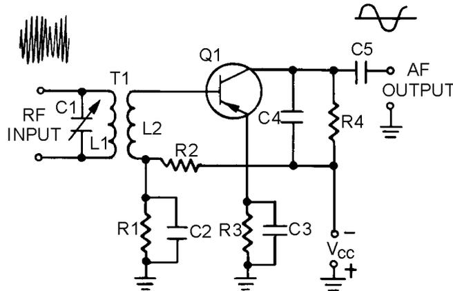
Figure 3-7.—Common-emitter detector.
