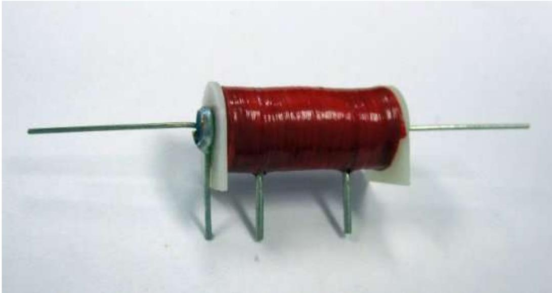
**Figure 11. A Typical Reed Relay with Electrostatic Guard Example**
