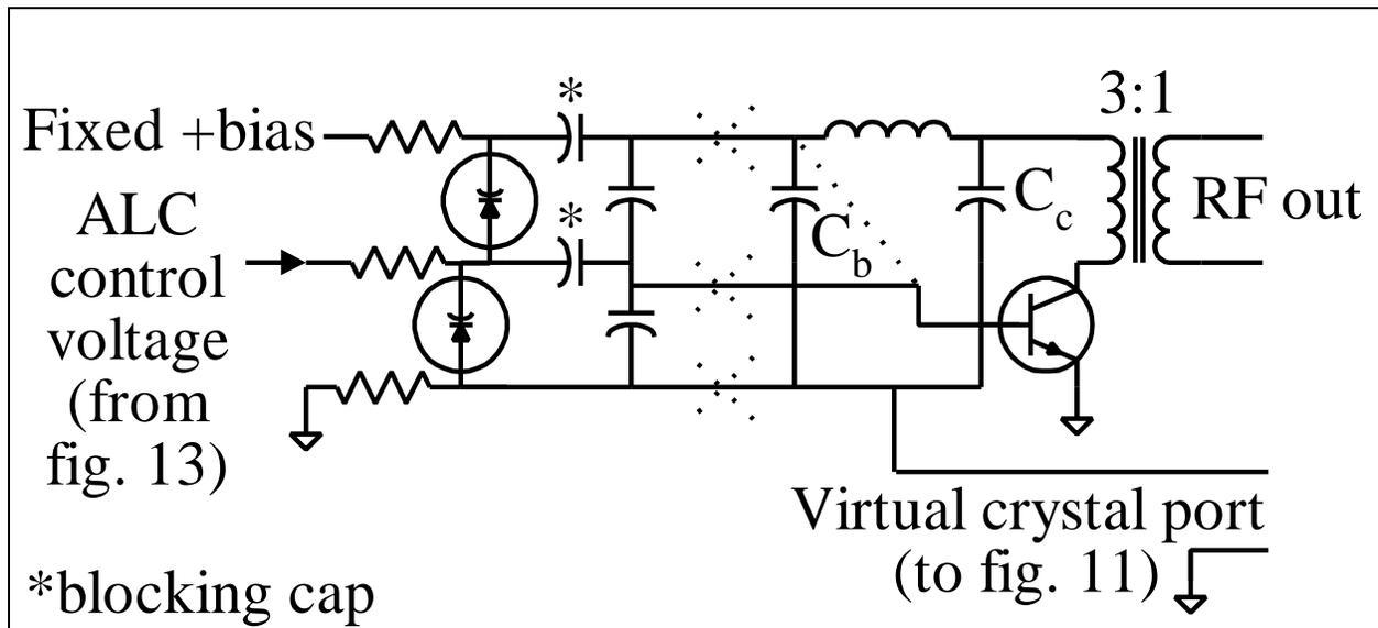
Figure 14. Bridged-T oscillator with gain control.
