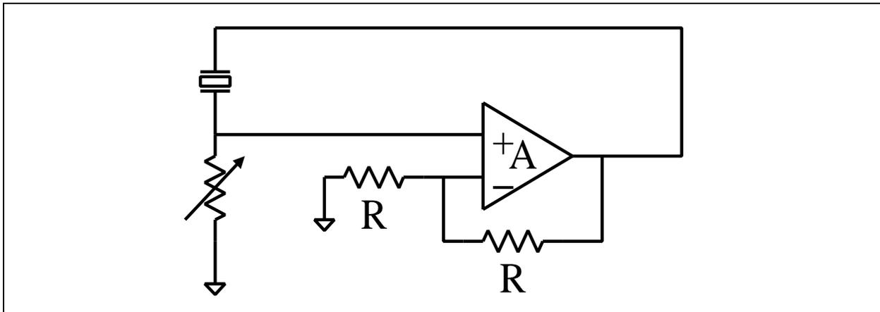
Figure 5. Meacham oscillator utilizing op amp.
