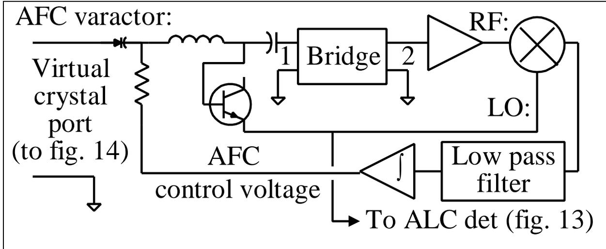
Figure 11. AFC system block diagram.
