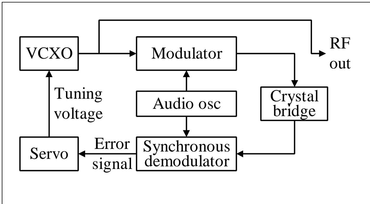
Figure 6. Bridge servo'ed oscillator.
