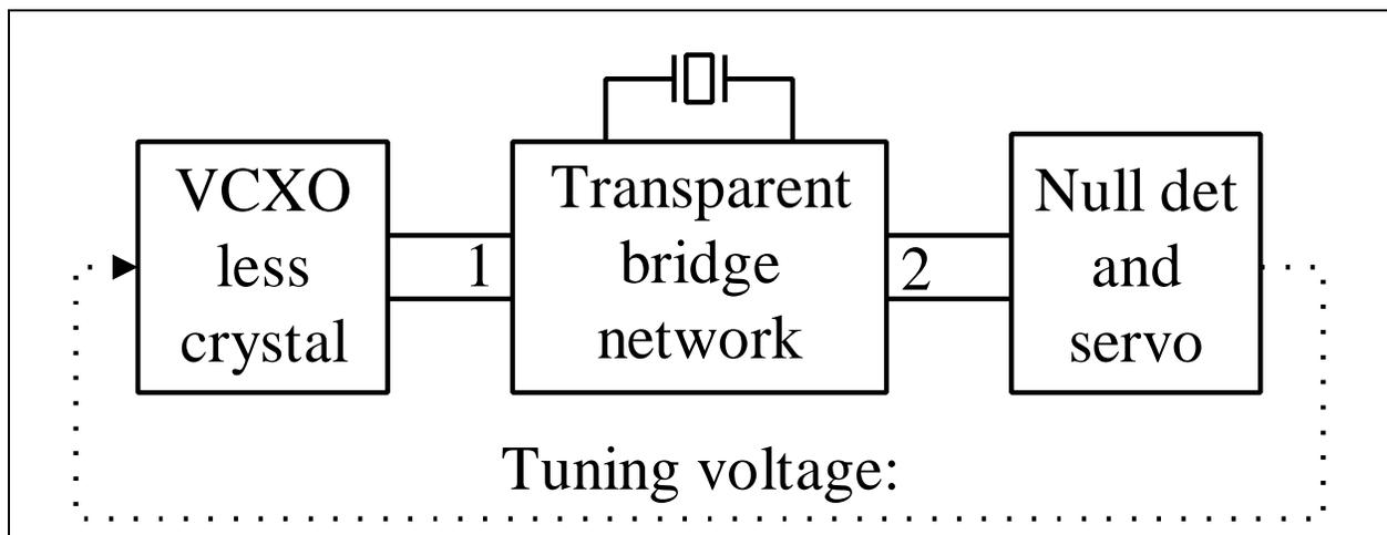
Figure 8. Balanced bridge controlled oscillator.
