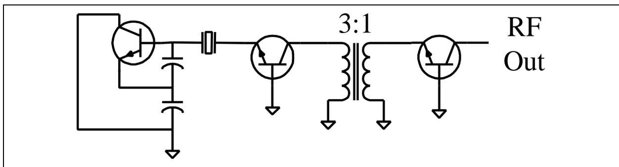
Figure 15. Burgoon low phase noise output circuit.
