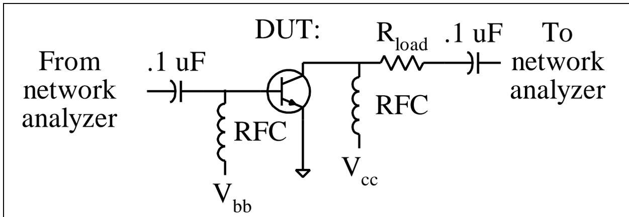
**Figure 3. Transistor tempco test fixture.**
