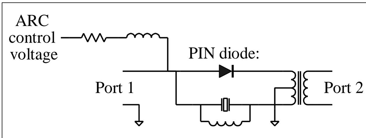
Figure 18. Adding ARC to bridge.
