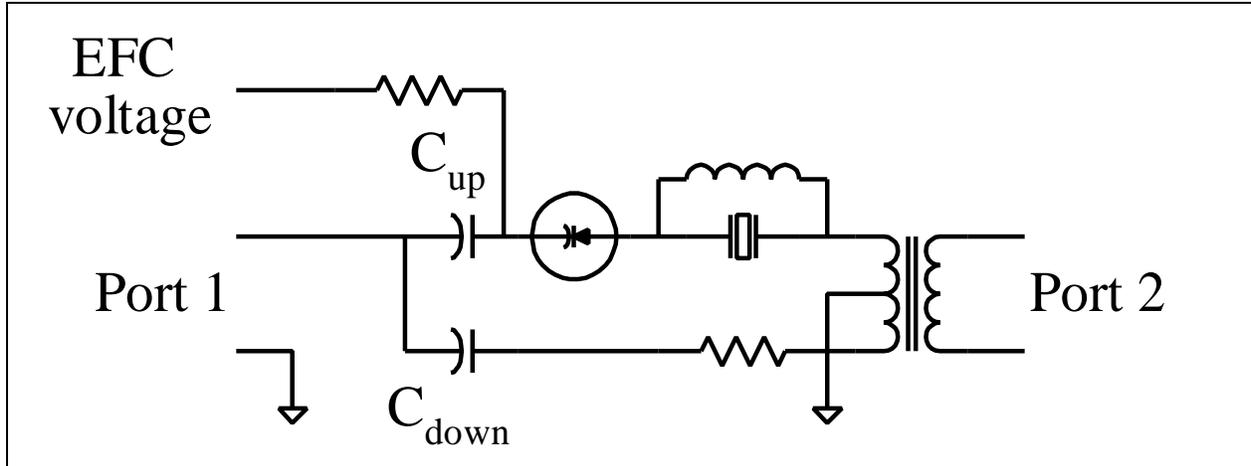
Figure 17. Adding EFC to bridge.
