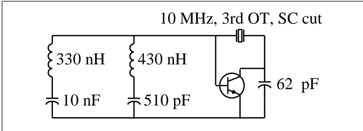
**Figure 2. Pierce oscillator with mode suppressor.**
