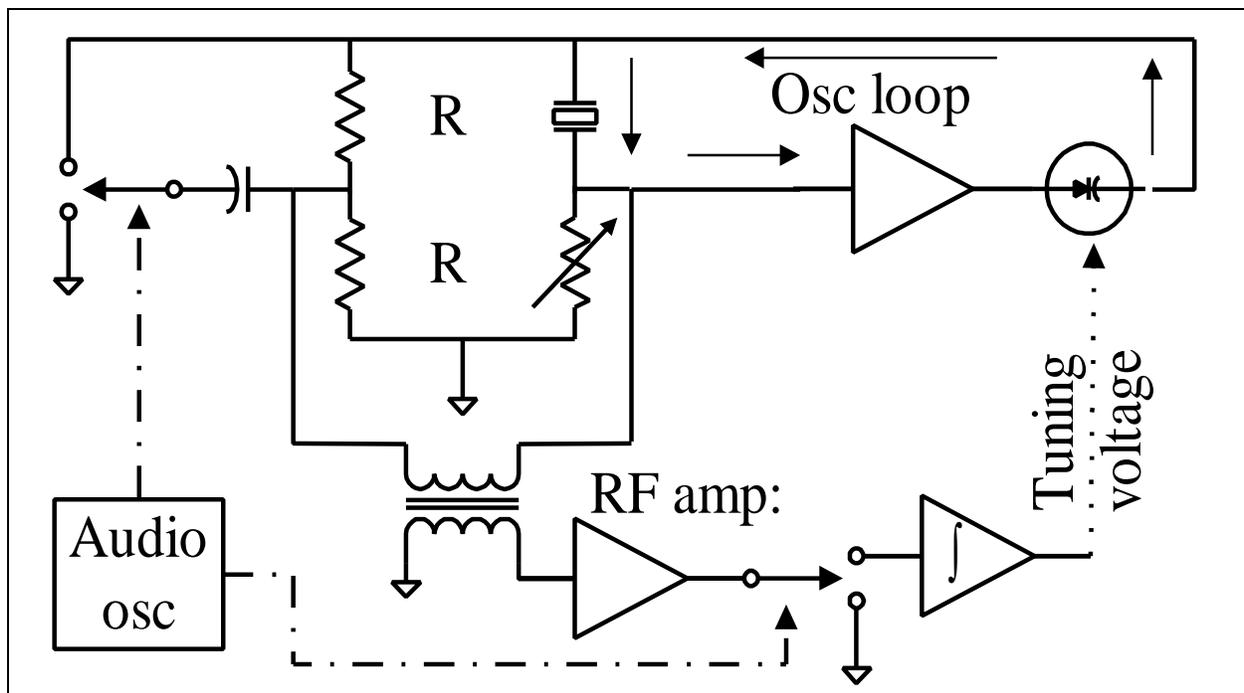
Figure 7. Sulzer bridge-balancing oscillator.
