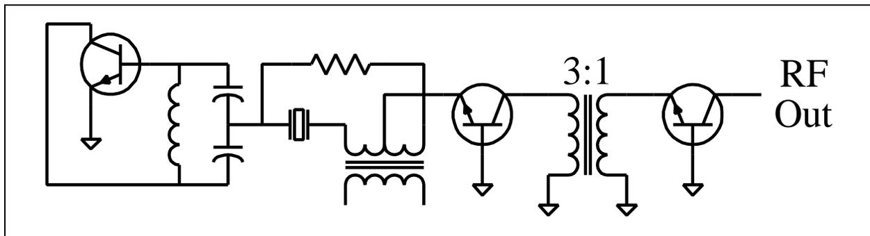
Figure 16. Output adaptation to bridge oscillator.
