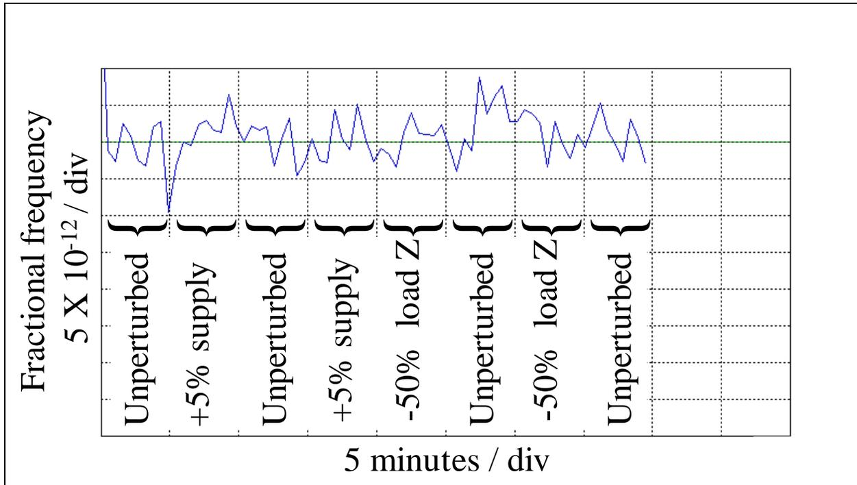
Figure 22. Power supply and load impedance effects.
