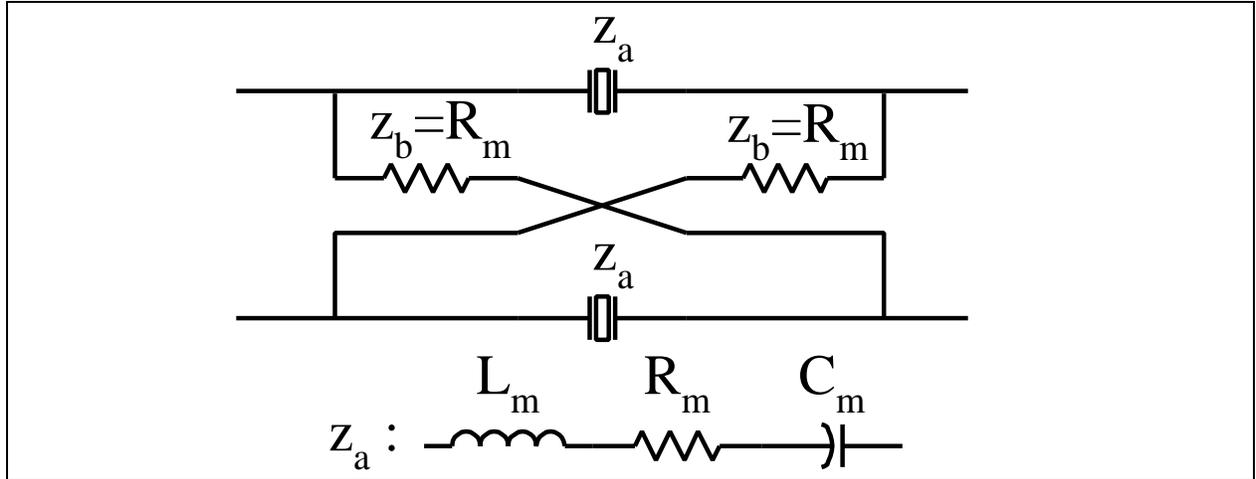
Figure 9. Theoretical transparent crystal bridge.
