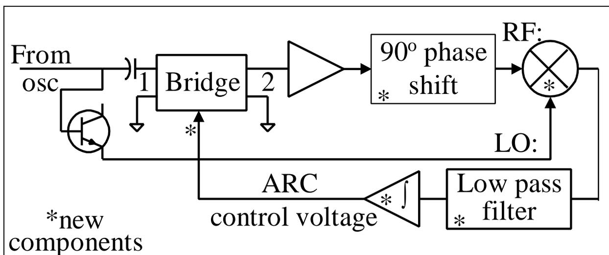
Figure 19. Automatic resistance control (ARC) loop.
