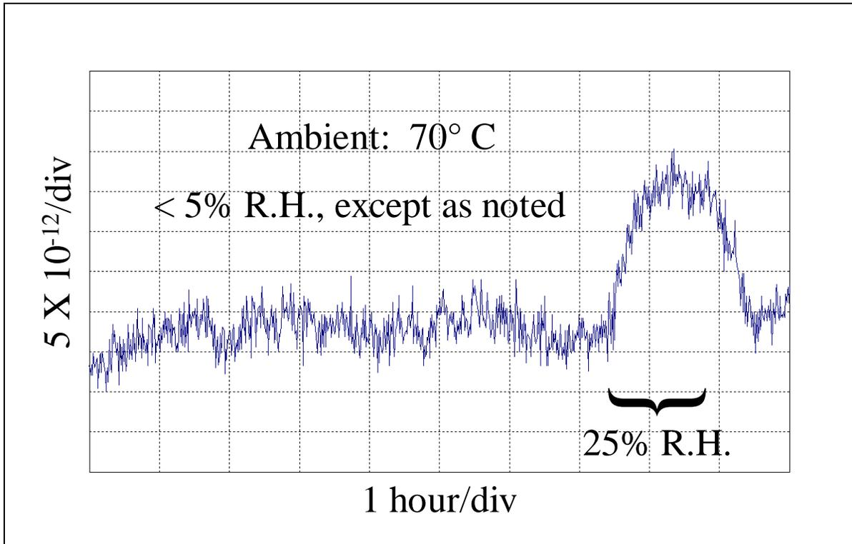
Figure 21. Effect of humidity on frequency.
