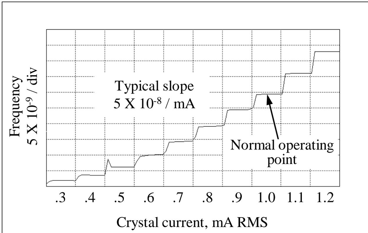
Figure 12. Drive level induced frequency shift.
