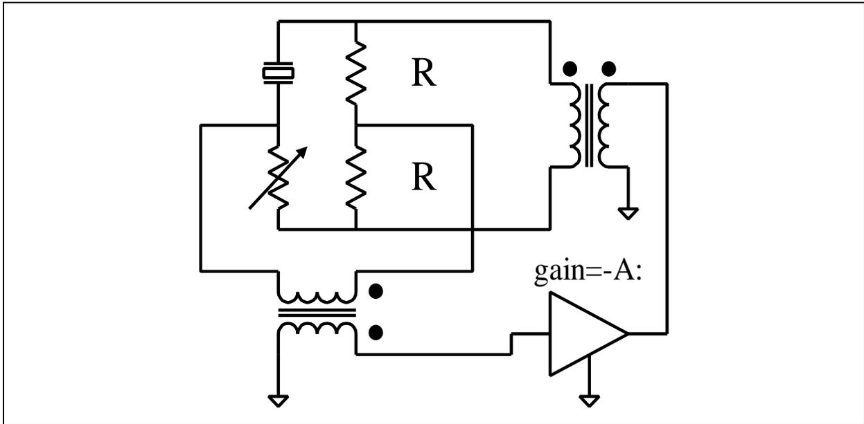
Figure 4. Meacham bridge-stabilized oscillator.
