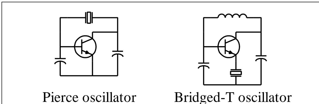
Figure 1. Basic oscillator circuits.
