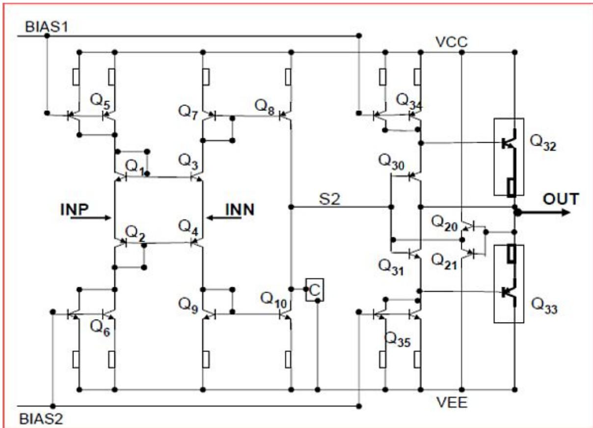
**Figure 2** IC design of one of the SCFAs of Figure 1
