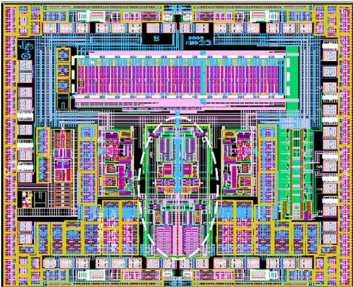
**Figure 5** A layout of a PGA containing the CFA, circled. The rest of the layout includes a R-2R switch array for the PGA, digital control and biasing circuits.
