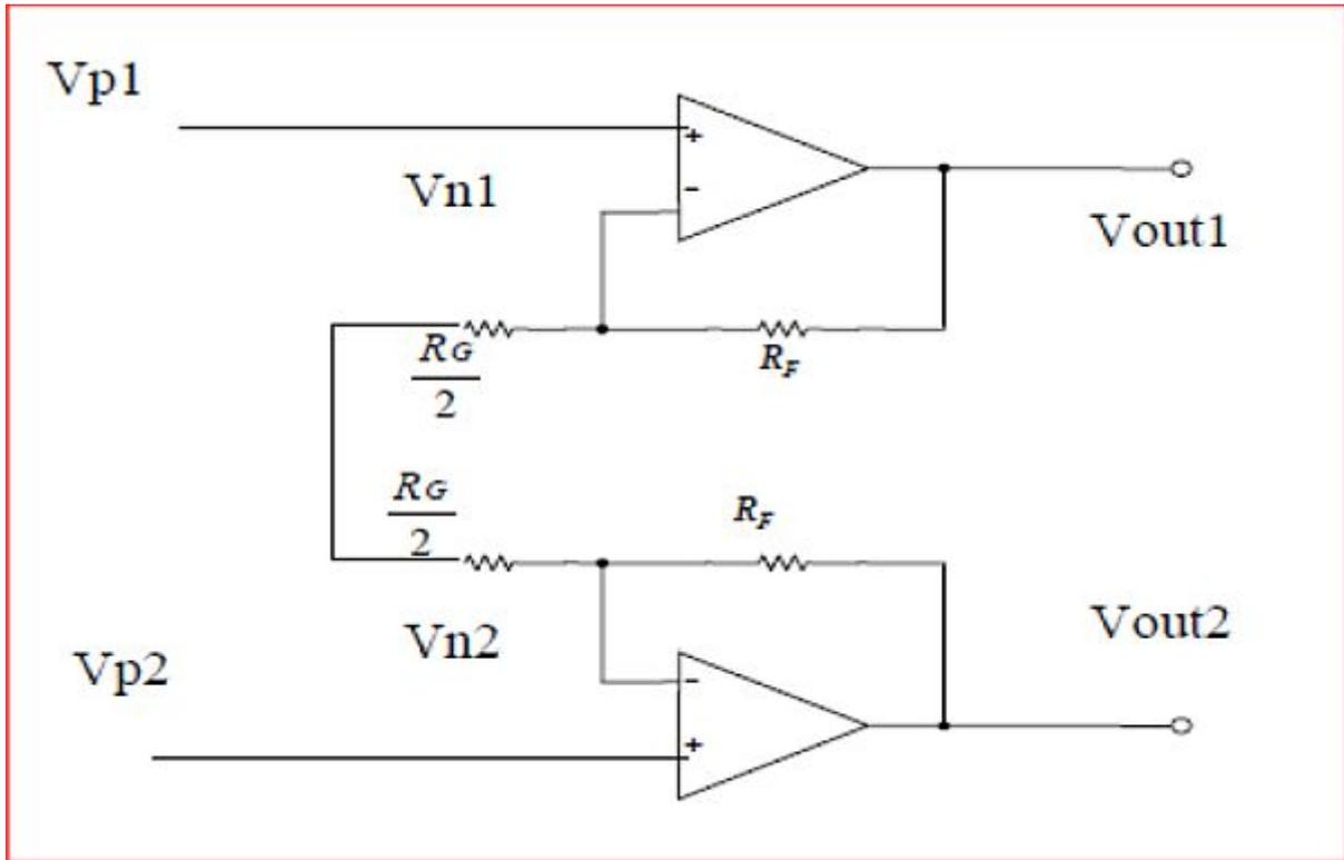
**Figure 1** The pseudo-differential amplifier CFA with two identical single-ended current feedback amplifiers (SCFA).
