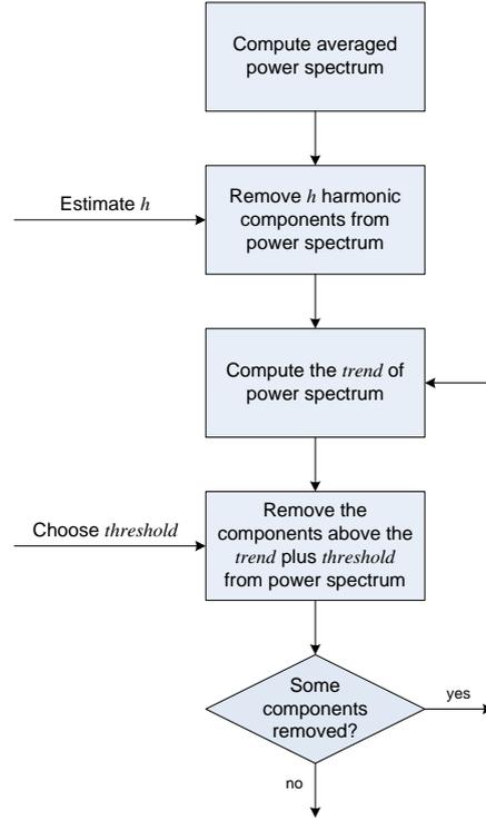
Fig. 2. Block diagram of the proposed algorithm
