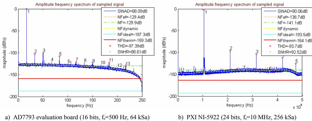
Fig. 3. ADC noise floors plotted in amplitude frequency spectra
