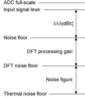
Fig. 1. Simplified diagram of noise floor levels
