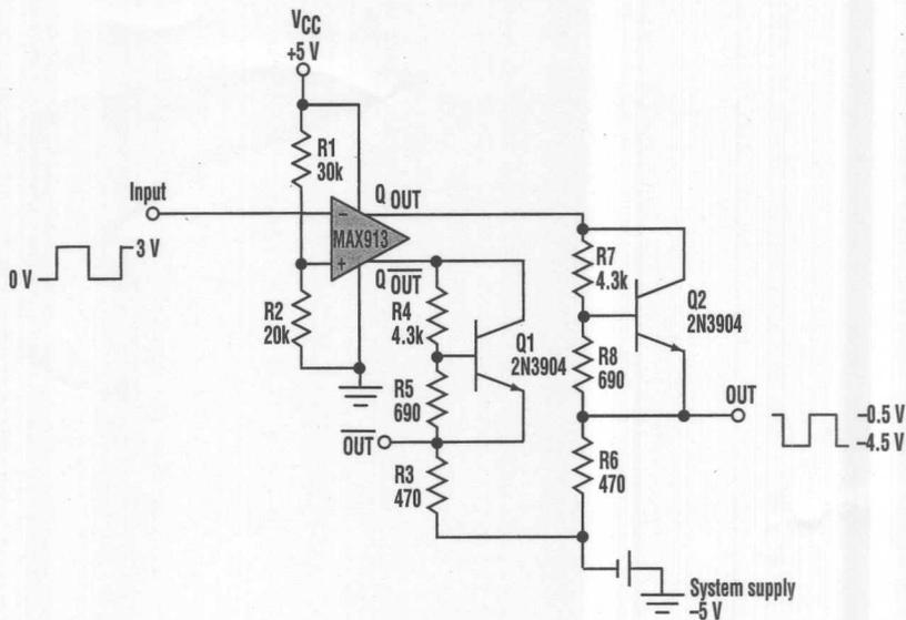
3. This circuit changes positive-going pulses to negative-going ones, while operating with a positive comparator supply and a negative system supply.
