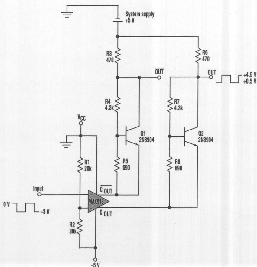
2. The circuit here translates negative-going pulses to positive-going ones, while operating with a negative comparator supply and a positive system supply.
