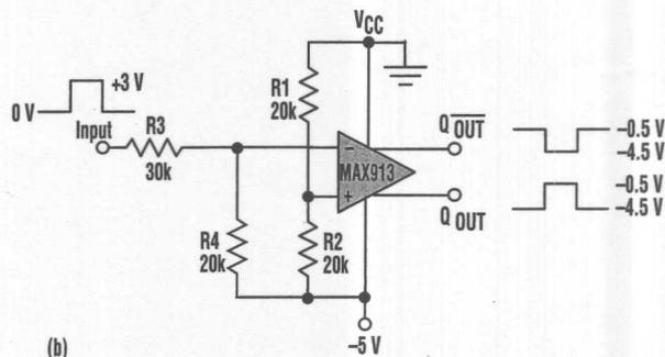
1. Operating from a positive supply, the circuit in (a) takes in negative input pulses and puts out complementary bipolar outputs. The circuit in (b) does just the opposite: It works off a negative supply and accepts positive input pulses to produce its complementary bipolar outputs.
