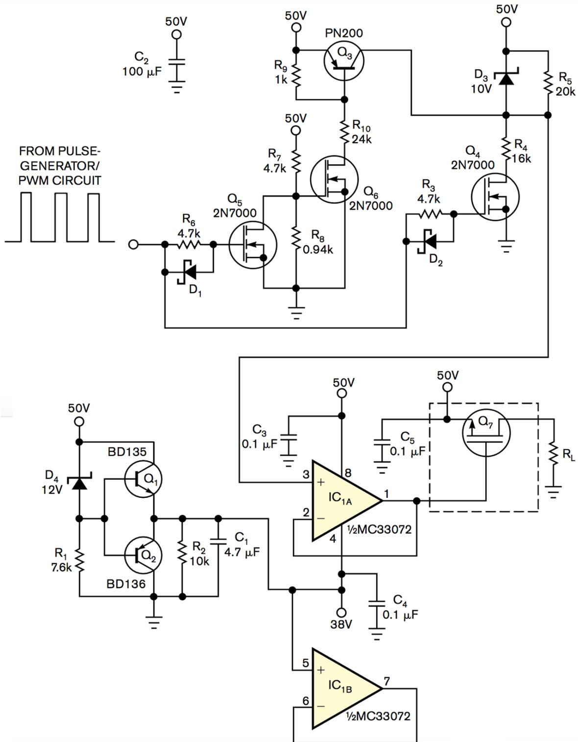
**Figure 1** An op amp operating at 38 to 50V provides power to a load through power-MOSFET Q<sub>7</sub>.
