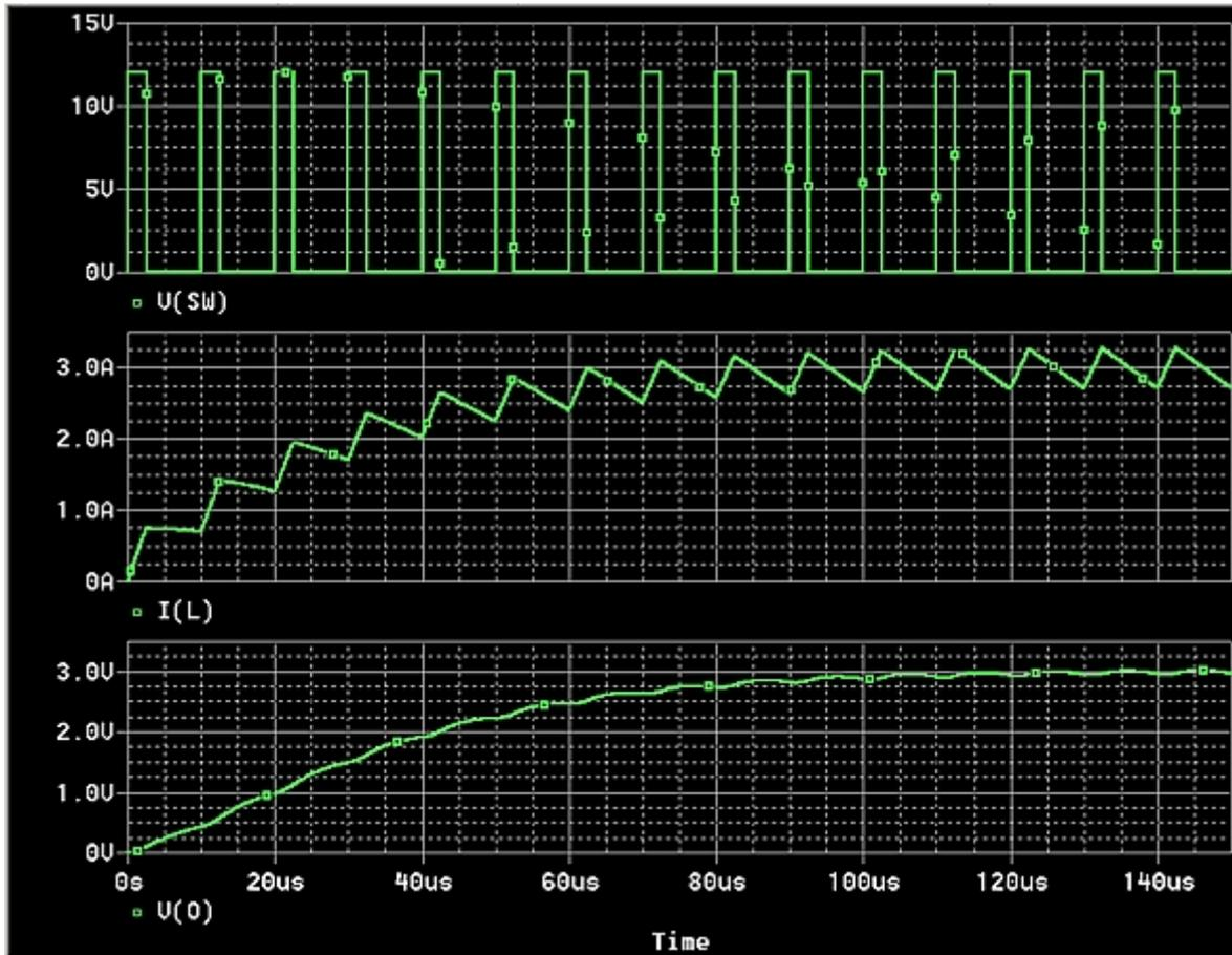
**Figure 2** PSpice waveforms for the circuit of Figure 1 for the case  $f_s = 100 \text{ kHz}$  and  $D = 0.25$ .
