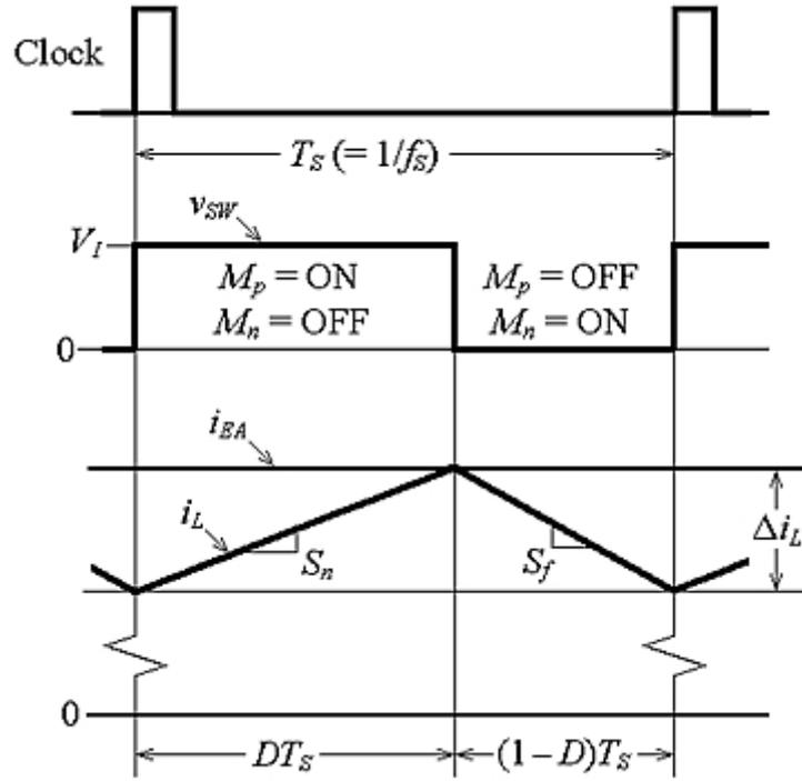
**Figure 4** Steady-state waveforms in peak-current-mode control (PCMC).
