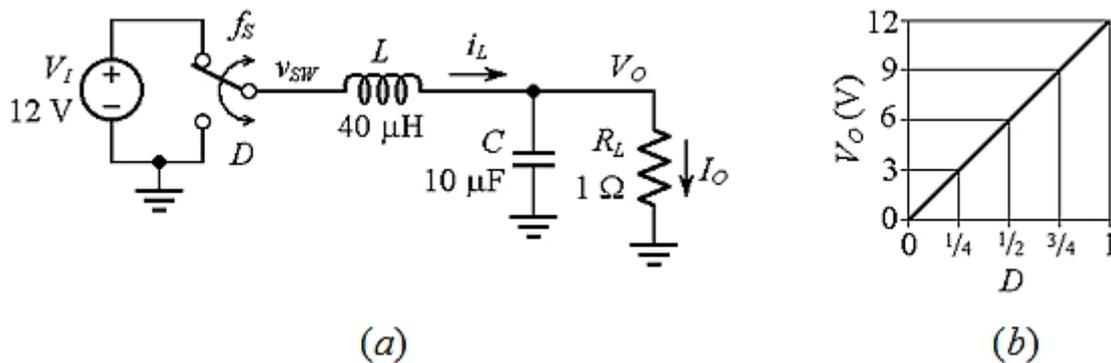
**Figure 1** (a) Buck conversion principle ( $f_s$  and  $D$  represent the frequency and duty cycle with which the switch is being toggled). (b)  $V_o$  as a function of  $D$ .
