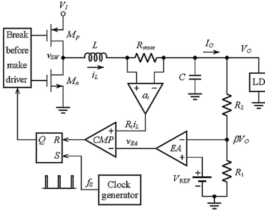
**Figure 3** Circuit schematic of a PCMC buck converter without slope compensation.
