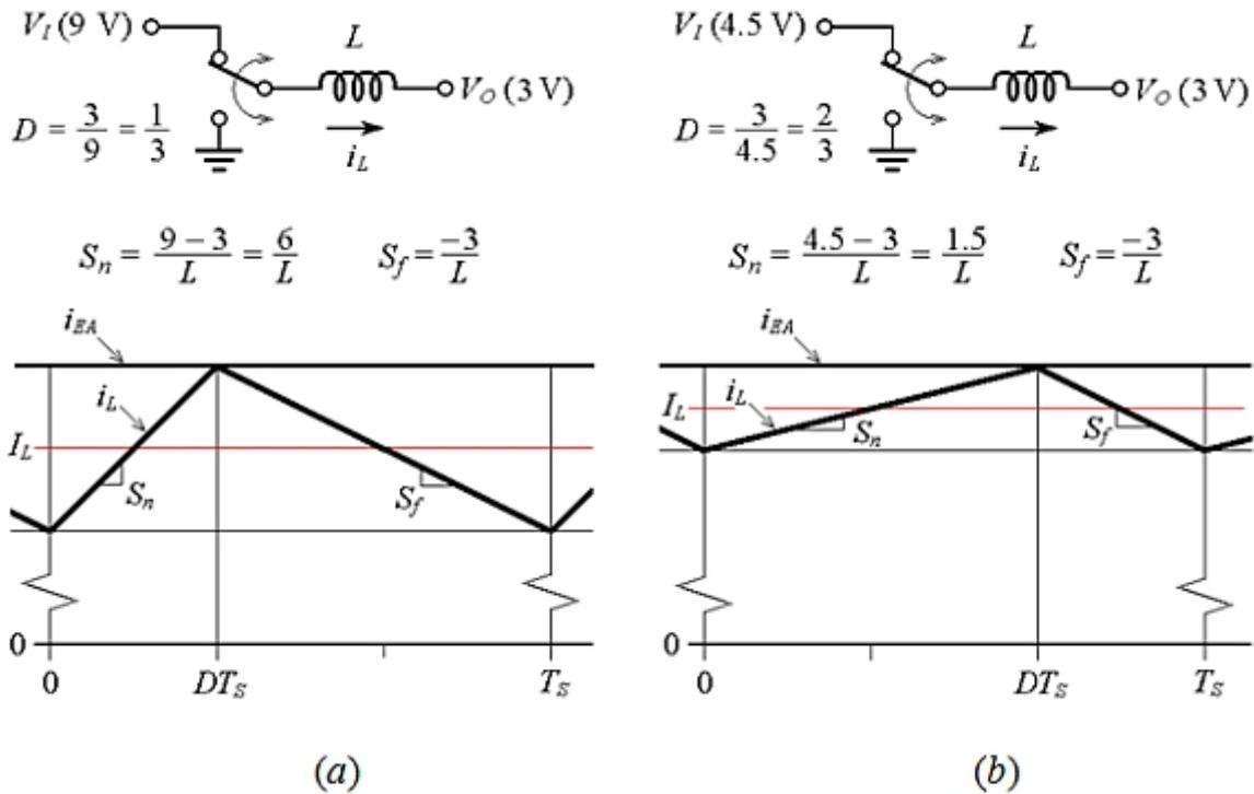
**Figure 5** The inductor current of the circuit of Figure 3 for two different duty cycles.
