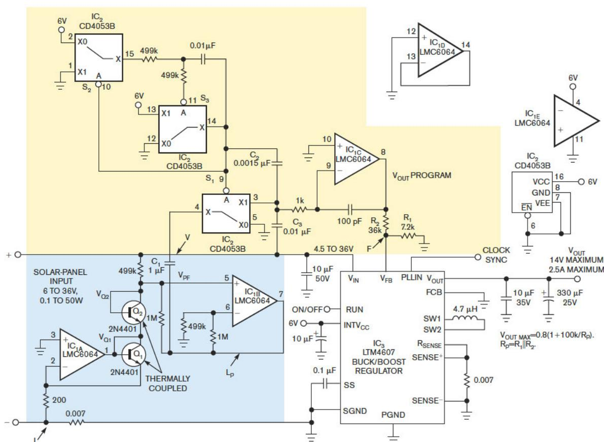
**Figure 2** This maximum-power-point-tracking controller relies on well-known logarithmic behavior of transistor junctions. (Click to enlarge)
