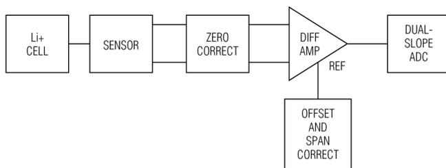
*Figure 1: Block diagram of the slope-ADC calibration circuit.*
