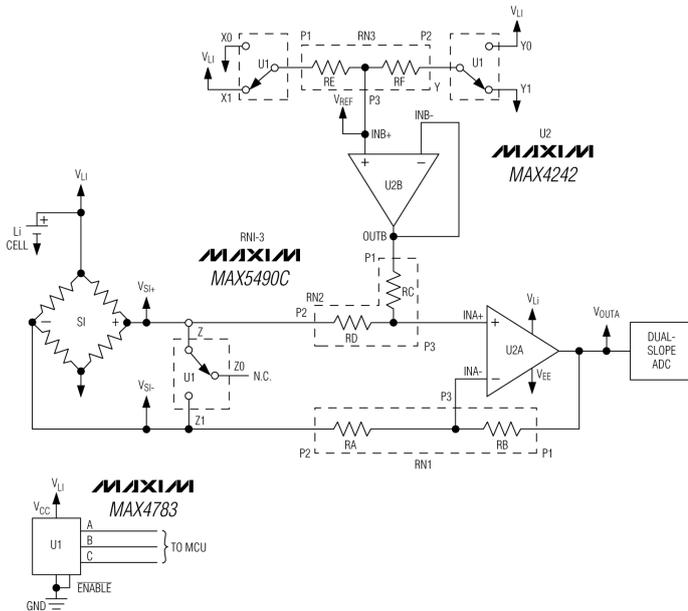
Figure 2: This circuit (depicted in Figure 1) produces offset and span readings, to be stored and used for on-the-fly calibrations of a dual-slope A/D converter (Click to enlarge image)
