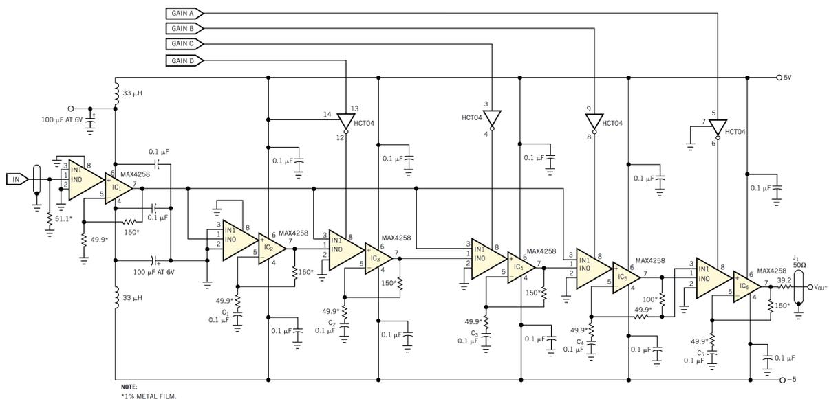
**Figure 1** You can obtain eight distinct gain settings with this low-noise, high-bandwidth video amplifier.
