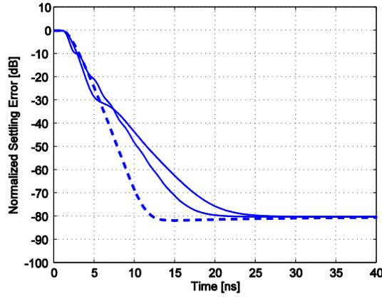
Fig. 7. The normalized settling error for  $f_a = 10.95$  MHz (dashed curve), 100 MHz, and 1 GHz with  $f_{p2} \approx 300$  MHz.
