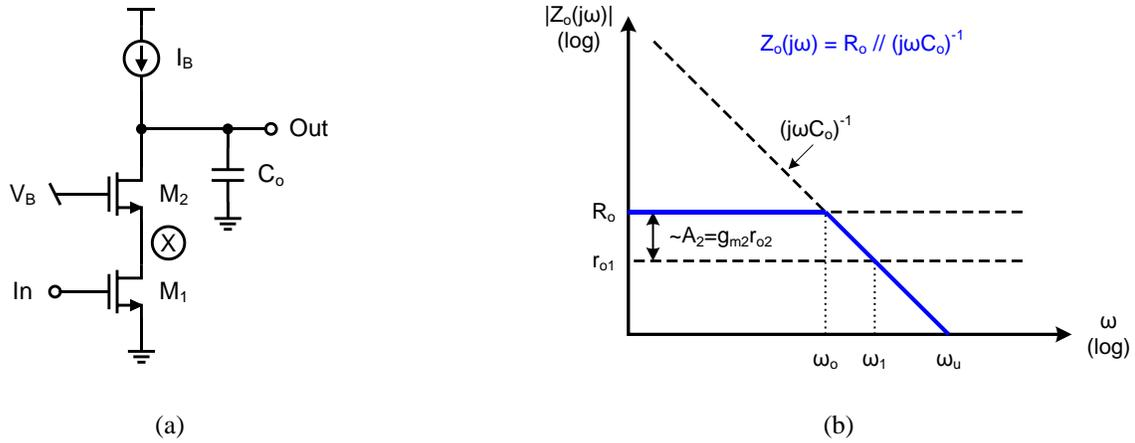
Fig. 1. CMOS cascode gain stage: (a) simplified circuit diagram and (b) Bode plot of the output impedance. The frequency dependence of the output impedance derives from  $C_o$ .
