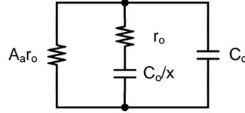
Fig. 3. Model of the output impedance of the active cascode in Fig. 2.
