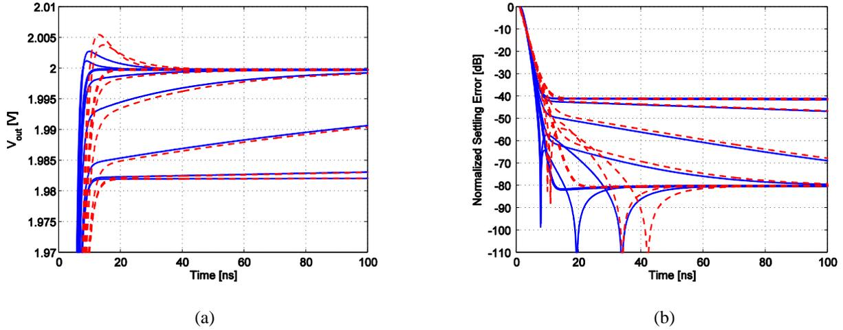
Fig. 5. The same results as those of Fig. 4 with the inclusion of  $C_m$ . The phase margin of the loop-gain is  $71^\circ$ . The dashed curves are for  $C_m = 0$ . The basic settling behavior remains the same in the presence of a second pole.
