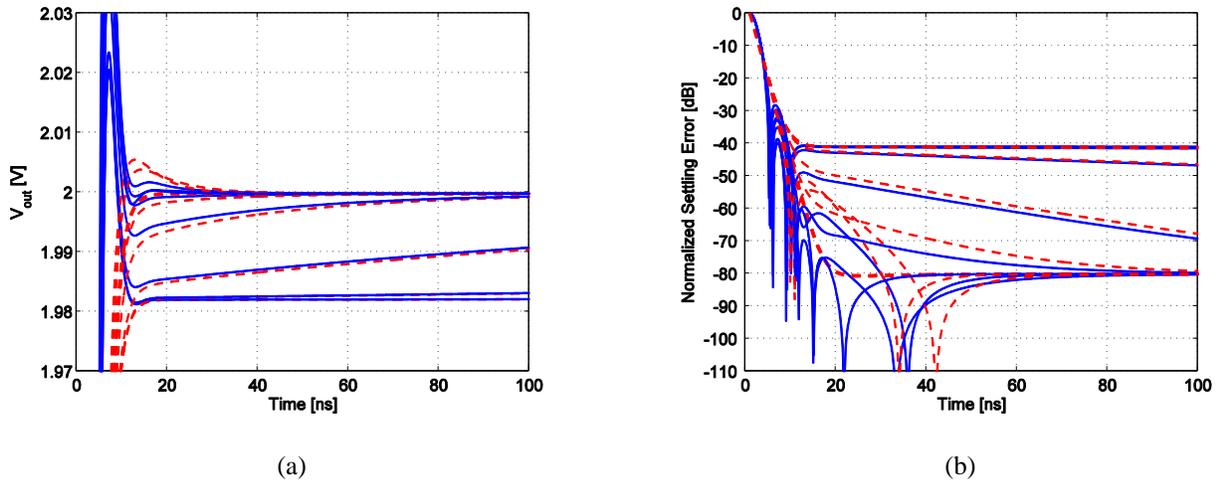
Fig. 6. The same results as those of Fig. 4 with the inclusion of  $C_m$  and the  $C_{gs}$ ' and  $C_{gd}$ 's of  $M_1$  and  $M_2$ . The slow tails of the transients closely resemble those of the original case (the dashed curves) in spite of the initial significant overshoots.
