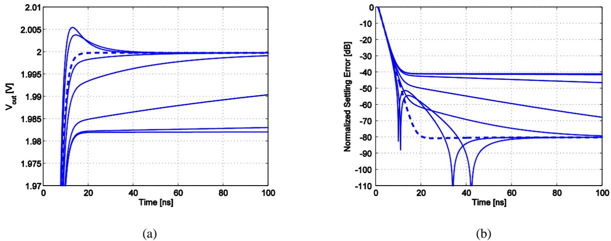
Fig. 4. Closed-loop settling behavior for  $f_a = 10$  kHz, 100 kHz, 1 MHz, 5 MHz, 9 MHz, 10.95 MHz, 20 MHz, and 30 MHz: (a) the amplifier output voltage (increasing in  $f_a$  from bottom up), and (b) the normalized settling error (increasing in  $f_a$  from top down). Open-loop parameters:  $f_a = 10$  kHz,  $f_u = 100$  MHz, and  $A_{o} = 80$  dB. The dashed curves ( $f_a = 10.95$  MHz) correspond to the case of  $k_2 = 0$ , i.e., exact pole-zero cancellation.
