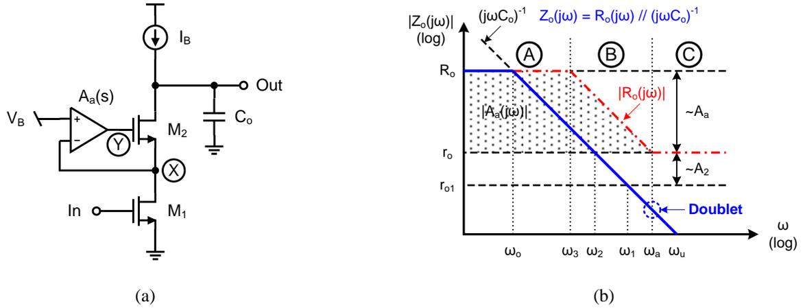
Fig. 2. CMOS active-cascode gain stage: (a) simplified circuit diagram and (b) Bode plot of the output impedance. The frequency dependence of the output impedance derives from  $C_o$  and the auxiliary amplifier  $A_a(s)$ .
