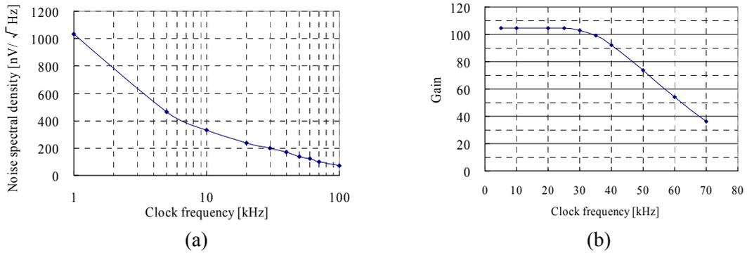
Fig. 7. Dependence on clock frequency: (a) noise spectral density; (b) gain of the circuit.
