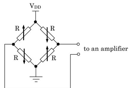
Fig. 1. A general structure of a piezoresistor sensor bridge.
