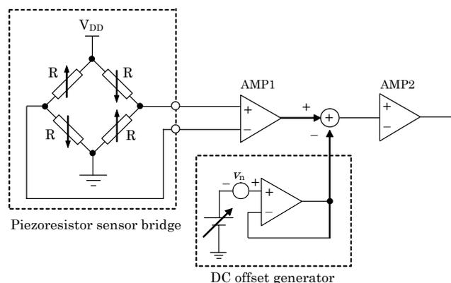
Fig. 2. Sensor-offset cancellation circuit.
