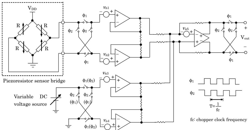
Fig. 3. Proposed circuit for sensor-offset cancellation.
