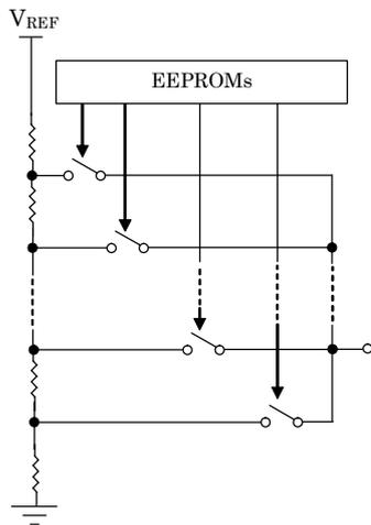
Fig. 4. A variable DC voltage source.
