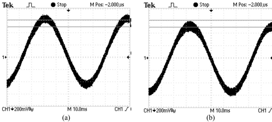
Fig. 9. Measured output waveform for a 15-Hz sinusoidal signal with an amplitude of 10mVpp and with a DC offset of 1mV: (a)  $in_2=in_3=0V$ ; (b)  $in_2=0V$ ,  $in_3=10mV$ .
