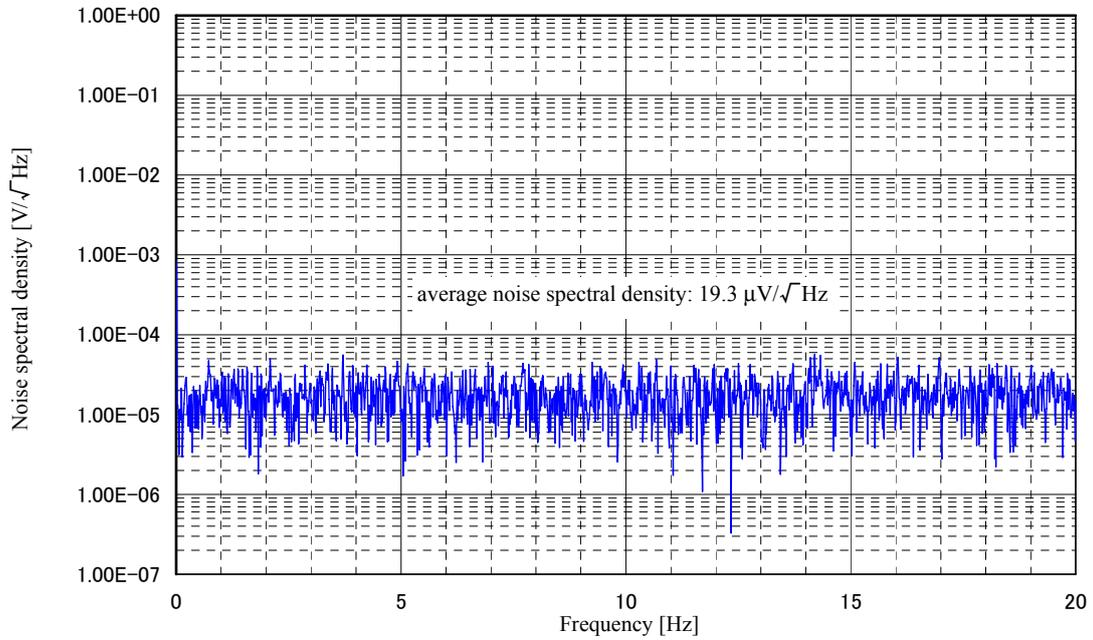
Fig. 8. Measured noise spectral density of the circuit (DC to 20Hz) with a 0-V input (x100 total gain).
