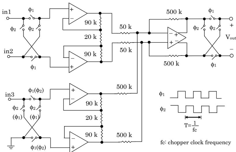
Fig. 6. Signal-conditioning circuit implemented in the chip.
