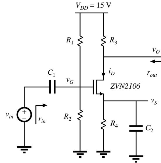
Figure 1: Discrete-circuit common-source amplifier.
