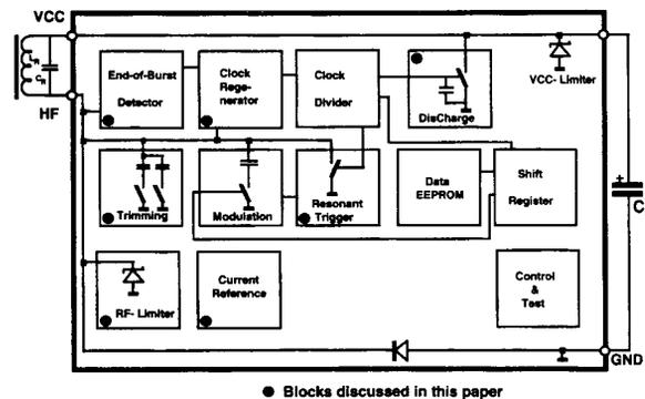
Fig. 2. Transponder block diagram.
