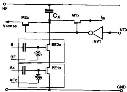
Fig. 12. EEPROM trim capacitor circuit.
