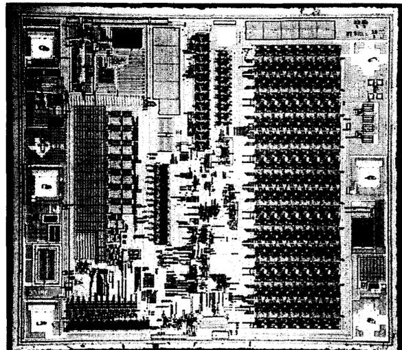
Fig. 13. Transponder chip photograph.
