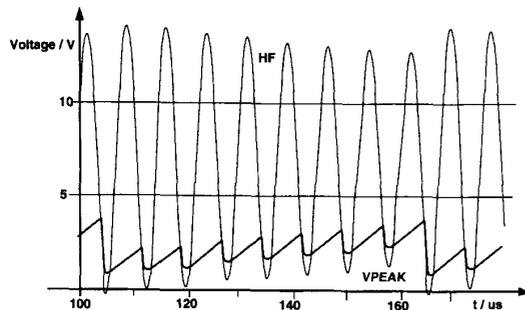
Fig. 9. Voltage in peak detector during transmission (pluck every eighth period).
