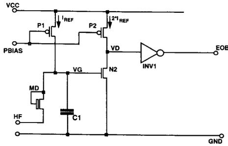
Fig. 5. End-of-burst-detector.
