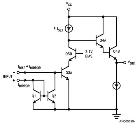
FIGURE 2. A simplified schematic of the LM359
