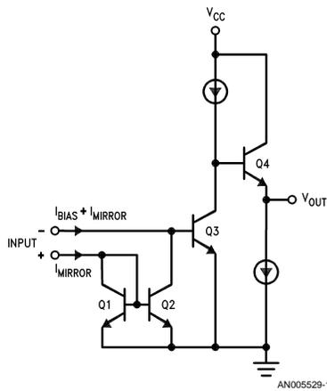
FIGURE 1. A simplified schematic of the LM3900
