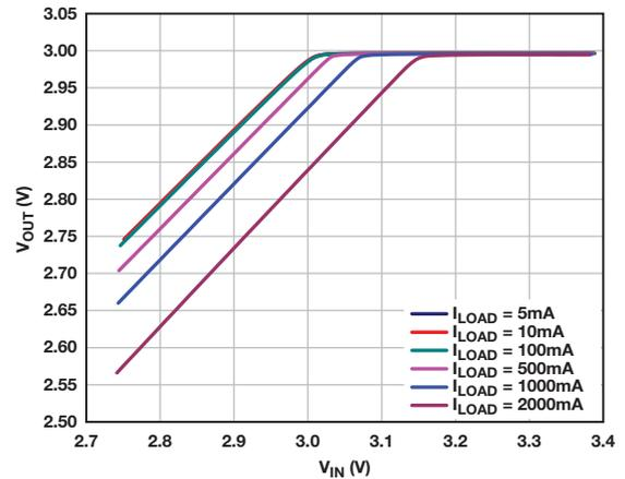
Figure 2. Dropout region of the 3.0-V [ADM7172](#) LDO.
