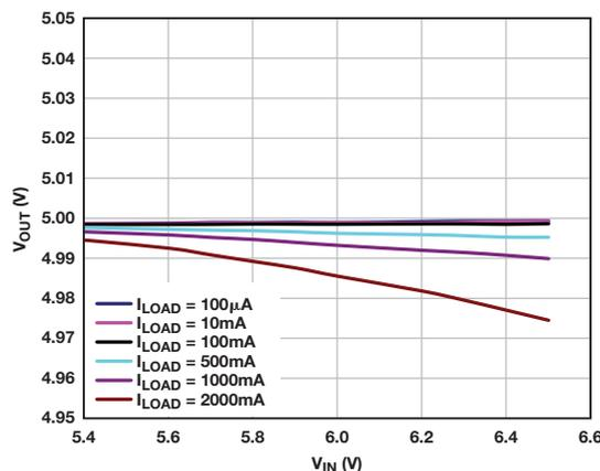
Figure 7. Output voltage vs. input voltage for the ADM7172 LDO.
