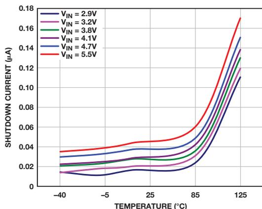
Figure 5. Shutdown current vs. temperature of the ADP160 LDO.
