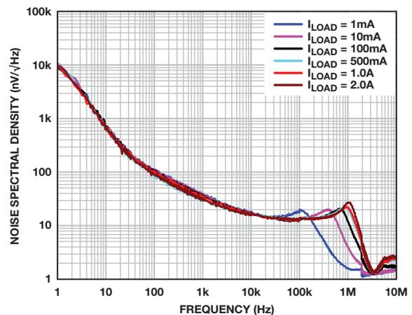
Figure 15. ADM7172 noise spectral density vs. load current.
