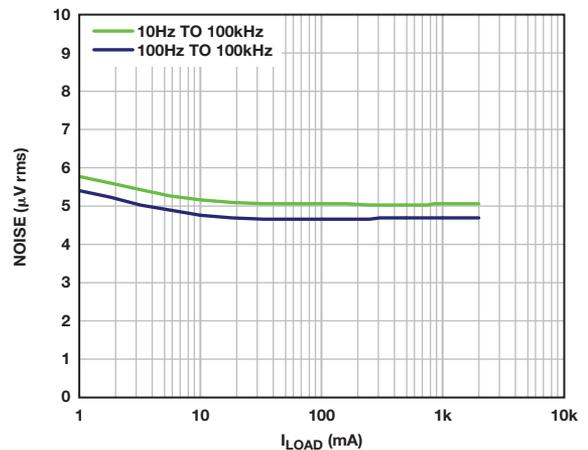
Figure 14. ADM7172 output noise vs. load current.
