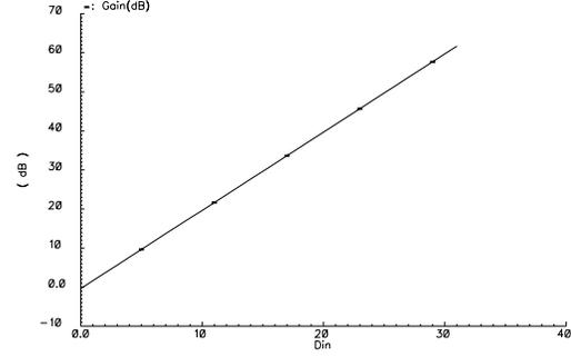
**Figure 9: The gain (in dB) of the VGA versus the input digital word**
