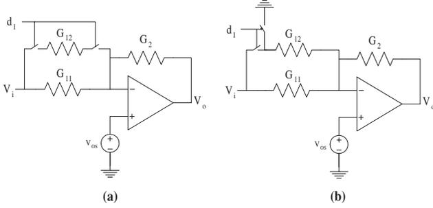
**Figure 2: (a) Conventional OpAmp-R VGA (b) Proposed constant-offset VGA circuit**
