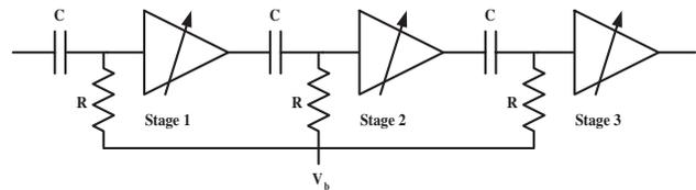
Figure 1: DC offset correction using passive HPF
