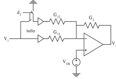
**Figure 3: Proposed constant-offset VGA circuit using OpAmp-R and passive HPF**
