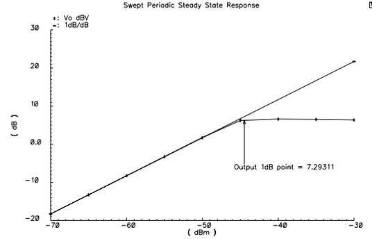
**Figure 10: 1dB compression curves for maximum and minimum gains**
