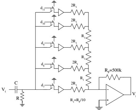
**Figure 8: Third stage VGA circuit**
