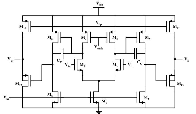
**Figure 4: 3-stage OpAmp schematic**
