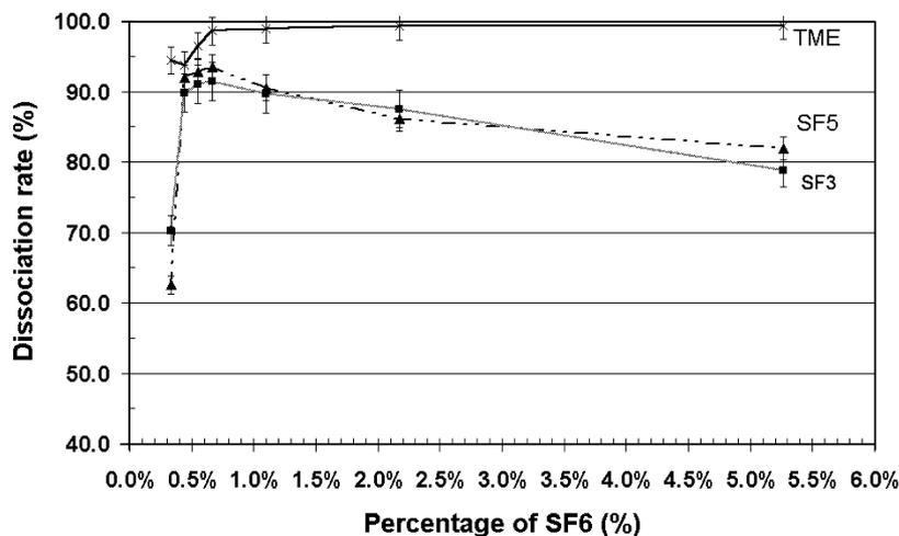
Fig. 3. Variation of the dissociation rates of TMT and SF<sub>6</sub> vs. percentage of SF<sub>6</sub> present in the gas mixture. (Experimental conditions: Ar–O<sub>2</sub>–TMT–SF<sub>6</sub> plasma; pressure: 15 Pa; Gas flow: 9 sccm; power: 190 W bias voltage: –120 V.)
