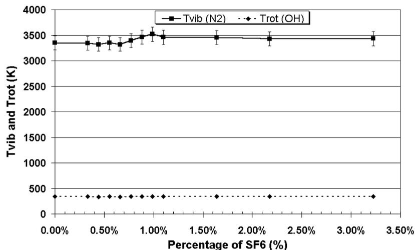
Fig. 2. Variation of the vibrational temperature of N<sub>2</sub> and Rotational temperature of OH with SF<sub>6</sub> flow rate. (Experimental conditions: Ar–O<sub>2</sub>–TMT–SF<sub>6</sub> plasma; pressure: 15 Pa; Gas flow: 9 sccm; power: 190 W bias voltage: –120 V.)
