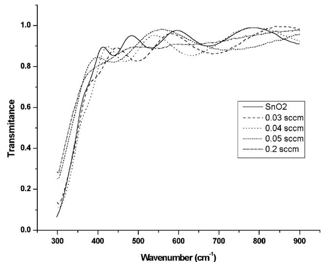
Fig. 8. Optical transmission curves. (Experimental conditions: Ar– $\text{O}_2$ –TMT– $\text{SF}_6$  plasma; pressure: 15 Pa; Gas flow: 9 sccm; power: 190 W bias voltage: –120 V.)
