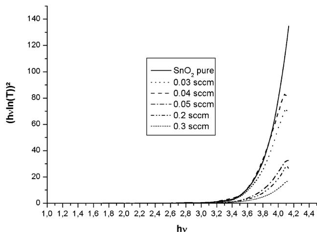
Fig. 9.  $(hv \log(T))^2 = f(hv)$  curves. (Experimental conditions: Ar–O<sub>2</sub>–TMT–SF<sub>6</sub> plasma; pressure: 15 Pa; Gas flow: 9 sccm; power: 190 W bias voltage: –120 V.)
