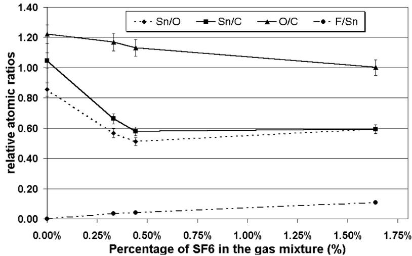
Fig. 5. Evolution of relative atomic ratios vs. percentage of SF<sub>6</sub> present in the gas mixture. (Experimental conditions: Ar–O<sub>2</sub>–TMT–SF<sub>6</sub> plasma; pressure: 15 Pa; Gas flow: 9 sccm; power: 190 W bias voltage: –120 V.)
