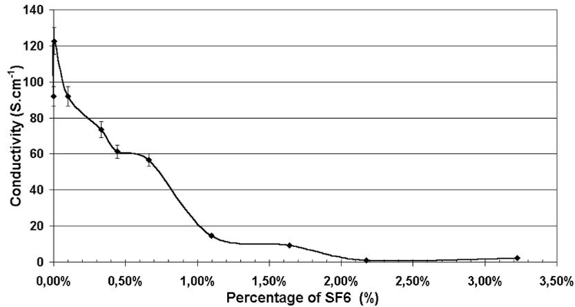
Fig. 1. Variation of the electrical conductivity with SF<sub>6</sub> flow rate. (Experimental conditions: Ar–O<sub>2</sub>–TMT–SF<sub>6</sub> plasma; pressure: 15 Pa; Gas flow: 9 sccm; power: 190 W; bias voltage: –120 V.)
