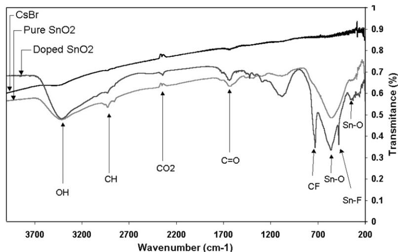
Fig. 6. FTIR spectra. (Experimental conditions: Ar–O<sub>2</sub>–TMT–SF<sub>6</sub> plasma; pressure: 15 Pa; Gas flow: 9 sccm; power: 190 W bias voltage: –120 V.)
