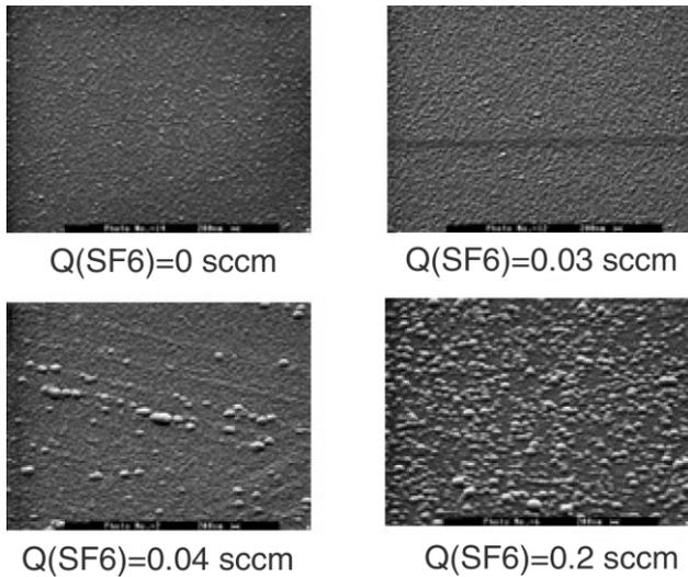
Fig. 7. SEM micrographs of tin oxide films doped by fluorine; role of  $\text{SF}_6$  flow rate. (Experimental conditions: Ar– $\text{O}_2$ –TMT– $\text{SF}_6$  plasma; pressure: 15 Pa; Gas flow: 9 sccm; power: 190 W bias voltage: –120 V.)
