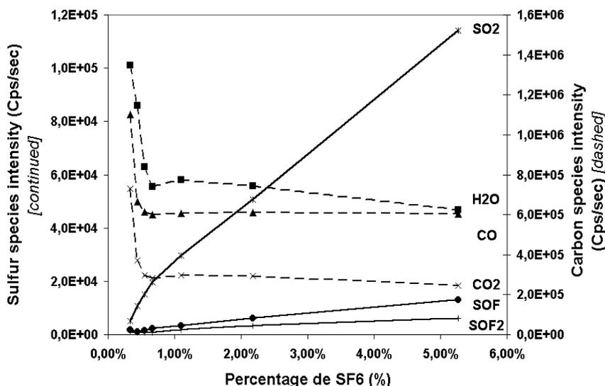
Fig. 4. Evolution of the intensities of identified species observed by MS as a function of SF<sub>6</sub> percentage introduced in the discharge. (Experimental conditions: Ar–O<sub>2</sub>–TMT–SF<sub>6</sub> plasma; pressure: 15 Pa; Gas flow: 9 sccm; power: 190 W bias voltage: –120 V.)
