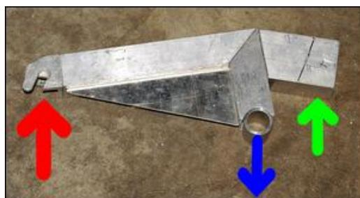
In operation, the arm is subject to the mostly upwards push of the wheel (red arrow), the downwards pull of the suspension bush (blue arrow), and the upwards push of the spring (green arrow)
